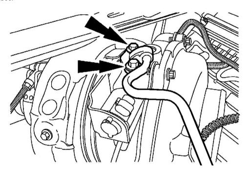
10. Remove the bolt and turbocharger oil supply tube. Remove and discard the O-ring.
