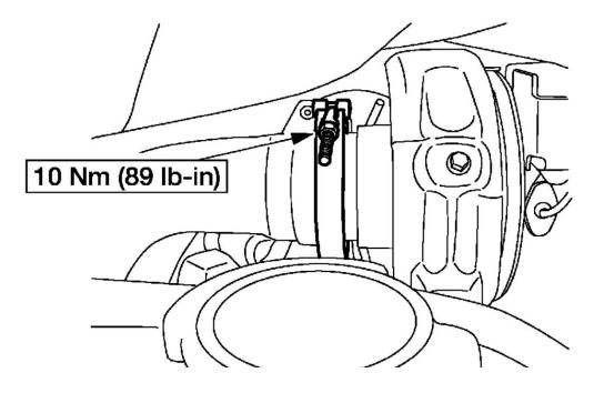
7. Install a new O-ring and apply clean engine oil. Install the oil supply tube. Position the locking bracket and install the bolt.
