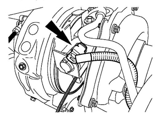
9. Remove the bolts for the oil supply tube. Remove and discard the gasket. IMPORTANT: If you have the old style oil feed line we recommend replacing it with the updated solid feed line Ford Part # 3C3Z-9T516-A. The old flex style feed line is known for damaging turbos.
