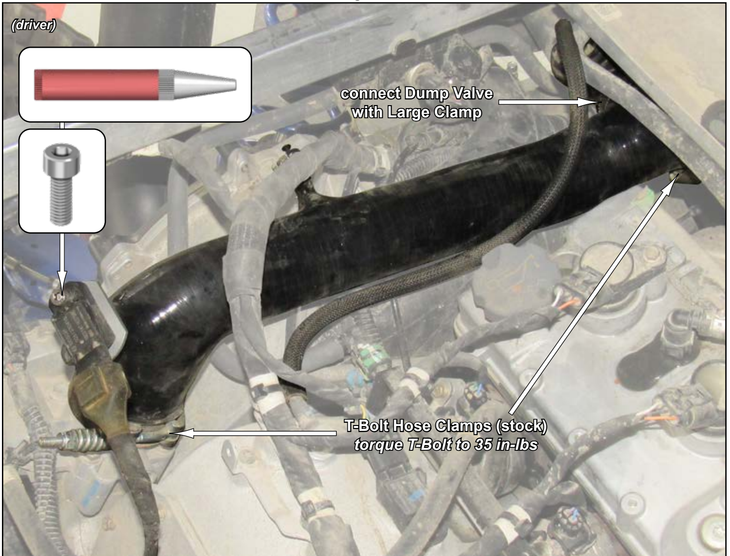
install new Charge Tube to machine
