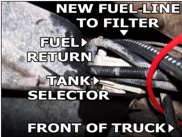
Figures 7a & 7b – Completed Tank Selector to Filter Head Plumbing
