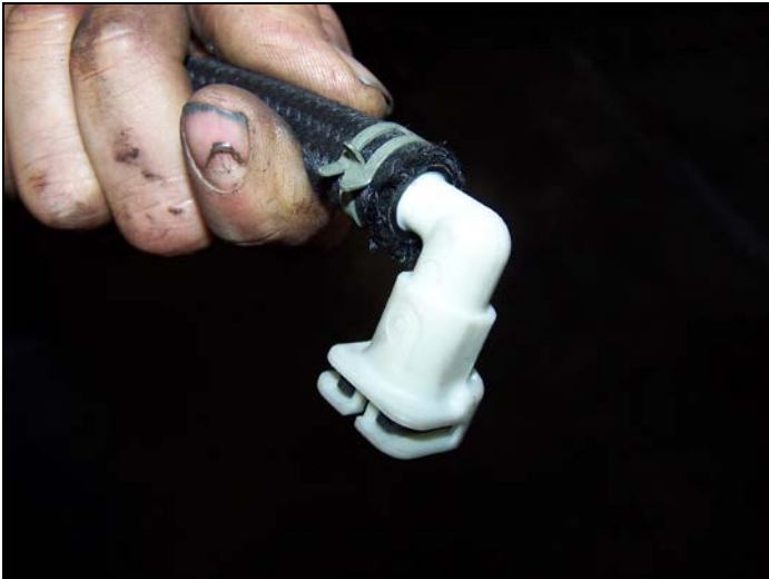
Figures 6a & 6b– Driven Diesel Quick Disconnect Fitting (left) and JIC Fitting (right)
