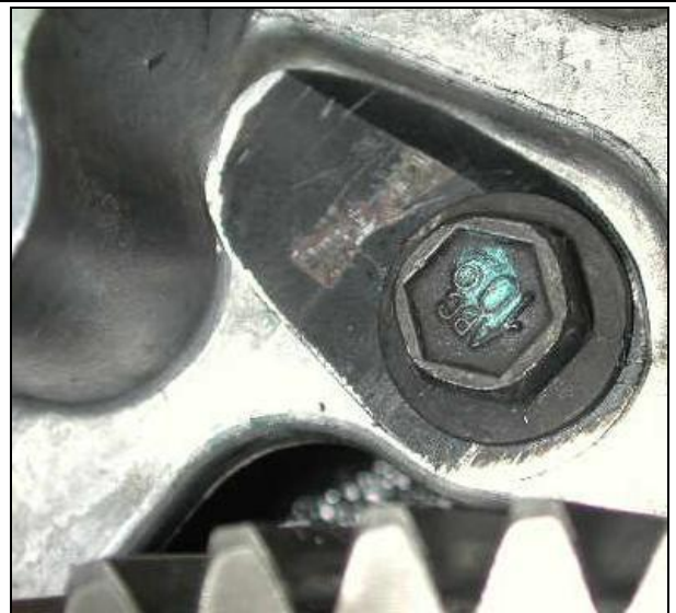
With retainer and bolt installed
