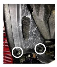
Fold back the rubber flap inbetween the front bumper and fender shown below. Carefully pull back the upper inner fender well to reveal the top of the fog light back splash. Repeat for passenger side.
