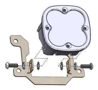
6. To install the Squadron assemblies, begin by placing one of the OEM screws through a hole in the bracket, then through the spacer. Move the assembly into position and then tighten the screw enough to hold it on the vehicle, but leave room for adjustment. Carefully place all the other spacers and screws and tighten partially. Adjust the light in the fog pocket opening until satisfied. Tighten. Repeat for opposite side of the vehicle.
