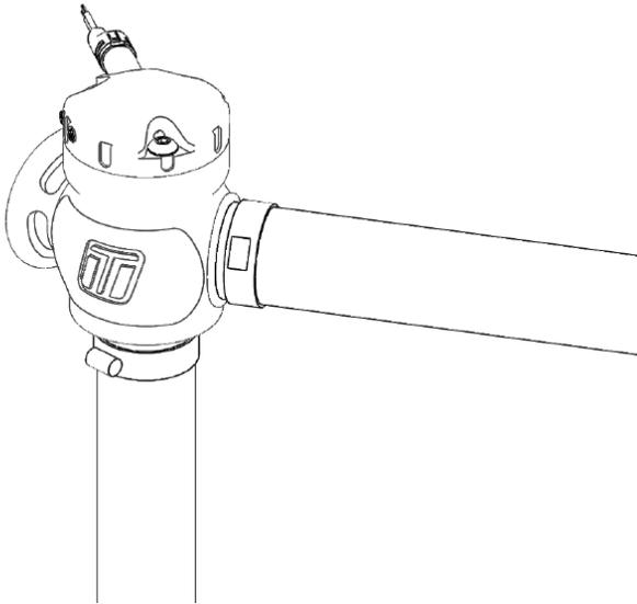
Once the valve has been mounted, connect the electrical plug into the OEM factory plug or into BOV controller and secure the wiring safely away from a heat source.
