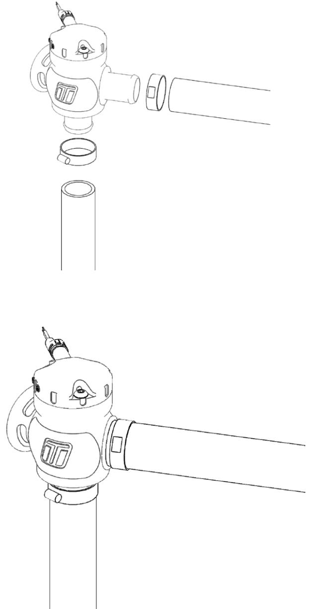
Once the valve has been mounted, connect the electrical plug into the OEM factory plug or into BOV controller and secure the wiring safely away from a heat source.
