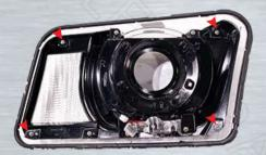
Remove these four T-10 Torx Screws first.
