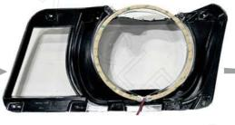
Place your ORACLE Halo ring right on top of the diffuser. Remove the 3M backing and make sure the wire is not in the way.
