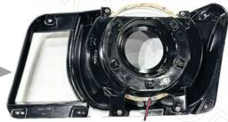
Re-install the Bezel and tighten down the four T-10 Torx
