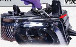
Use a flat head screwdriver to softly seperate the lens and the housing. Continue all the way around the headlight until it begins to part.
