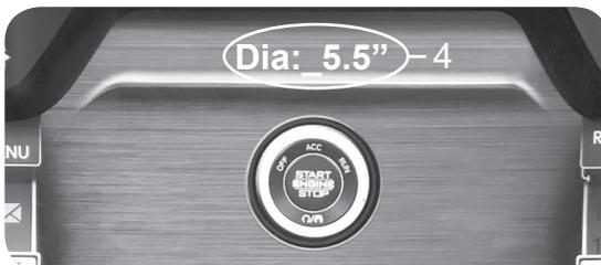
**STEP 6** - Use the accelerator pedal to adjust the number value, then press the SET+ button to select the displayed value.
