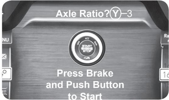
**STEP 4** - Use the accelerator pedal to adjust the number value, then press the SET+ button to select the displayed value.
