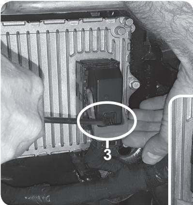
**STEP 4** - Once the lever is released, lift it upward until it stops. Disconnect the connector from the ECM.
