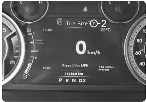
**STEP 1** - With the ignition in the RUN position (Do Not Start), press and hold the CANCEL (Cancel) button for approximately 5 seconds. *The option to modify the Tire Size is displayed.*
