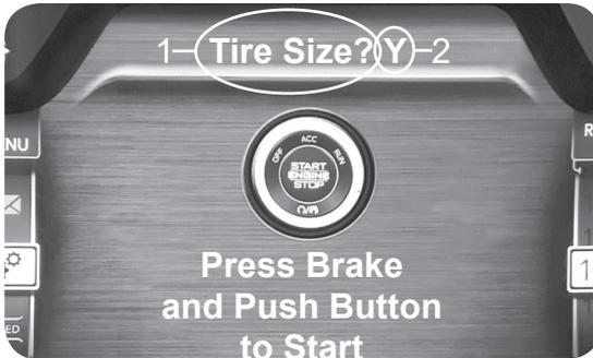
**STEP 2** - Press down on the accelerator pedal to change the N (No) to Y (Yes).
