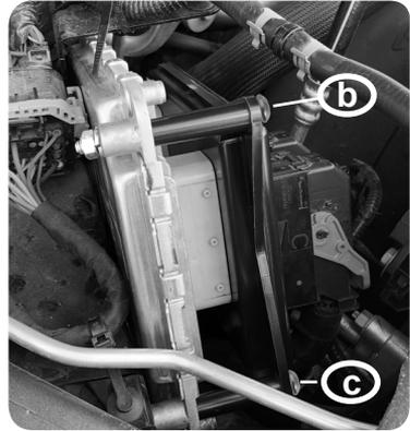
**STEP 12** - Gently insert the truck harness connectors into the Pulsar connectors. Push the lever down until it locks into place.
