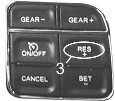
**STEP 3** - While the Y (Yes) is displayed, press the RES+ steering wheel button to select the option.
