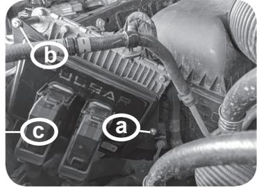
**Step 10** - Insert supplied bolts w/ washers into holes **(a)** and **(c)**, tighten with the provided Allen Wrench until snug.
