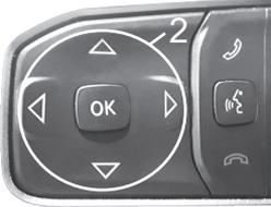
**STEP 2** - Using the left side steering wheel controls, enter the Screen Setup menu.
