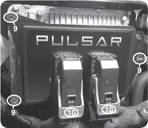
**STEP 10** - Gently insert the truck harness connectors into the Pulsar connectors. Push the lever down until it locks into place.
