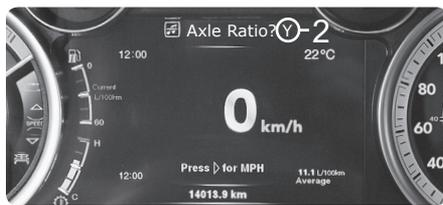
**STEP 2** - Press down on the accelerator pedal to change the N (No) to Y (Yes).
