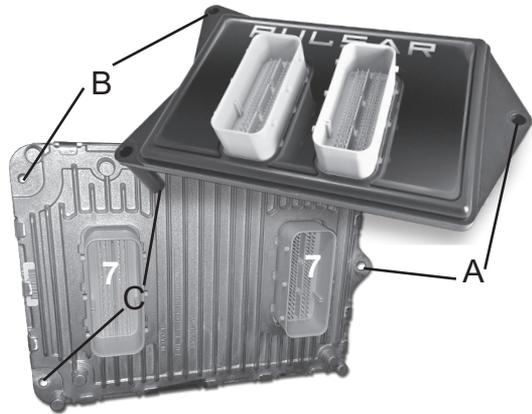
**STEP 7** - Align and insert the Pulsar's bottom side connectors with the ECM connectors.
