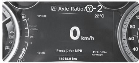
**STEP 2** - Press down on the accelerator pedal to change the N (No) to Y (Yes).
