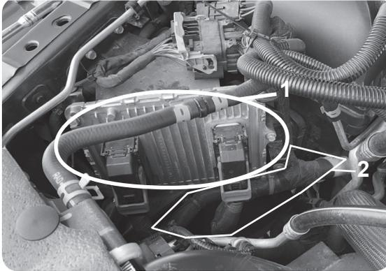
Cut the zip ties that fasten each connector harness to the metal bracket.
