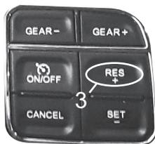
**STEP 4** - Use the accelerator pedal to adjust the number value, then press the RES+ button to select the displayed value.
