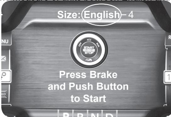
**NOTICE:** *If using English units, the value for the tire size should be set to the total height of the tire, not the rim (from the floor to the top of the tire).*
