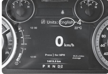
**STEP 5** - With the desired units displayed, press the RES+ button to select the Unit.
