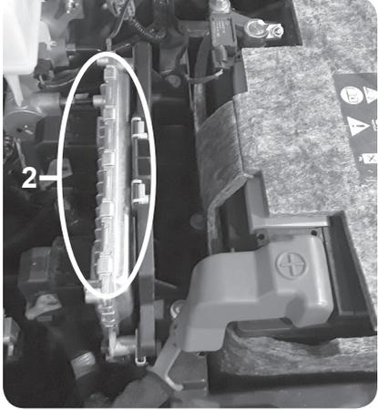
**STEP 3** - Use a flat head screw driver to press the lever lock towards the ECM. Gently lift up on the lever until you feel the lever release.
