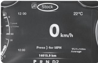
**NOTE:** When using MDS-OFF options, the dash display will show as if using manual gear shifting. This is to allow the Pulsar to control MDS, and **does not** actually put the vehicle into Manual Gear Shifting. When using an 8 speed transmission, it will automatically switch to gear 8. And when using a 6 speed transmission, it will automatically switch to gear 6.
