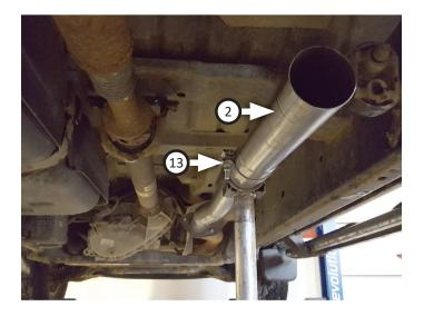
Place clamp (13) onto muffler (3) then connect it to inlet/extension pipe. Tighten clamp just enough to allow for adjustment then place (x2) clamps (13) onto muffler outlets.
