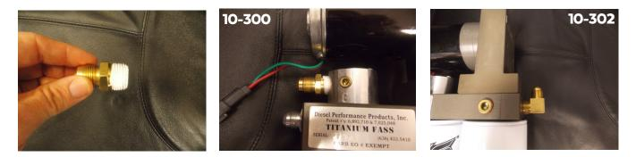
B. For fitting purposes. Secure PBR-2001 to pump assembly lightly with (3) 1/4"-20x1 3/4 bolts and (3)WA-1001D. This will assembly will be used in future steps for correct fitting of brackets. (Note:Bracket maybe flipped to accommodate your application.)
