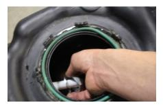
L. Carefully re-install pick up module. Do not bend Fuel Level float.
