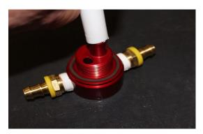
J. Place the suction tube assembly into hole. Take measurements so the bottom of the suction tube is only 1/8" (no more than 2 quarters stacked) from the bottom of the fuel tank. Before cutting the suction tube, triple check the measurements. It is more efficient to cut the tube too long and then correct to proper length than it would be to cut too short.
