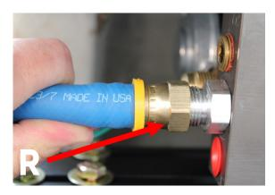
**C.** Insert PL-1005 in remaining fuel line using oil. Connect to the 'E" port of the FASS system. Torque to 18 ft./lbs. Route this fuel line to the factory fuel line feeding the engine. This fuel line is located be-hind the fuel cooler, discussed in Step 2c.
