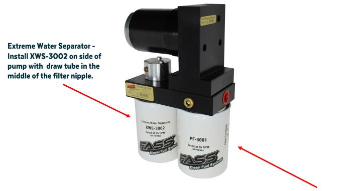
Particulate Filter -Install PF-3001 on filter nipple without the draw tube. Make sure to insert O-Ring provided on nipple.
