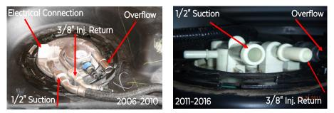
**F.** Remove the lock ring on top. Remove Fuel Module. Be careful not to bend the Fuel Level float. Now is a good time to find a cap to cover the 1/2" suction port on the Fuel Module. Choose location of BHF assembly
