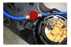
**N.** Reinstall fuel tank. Remember to reconnect factory suction, factory return line, and electrical harness. Torque tank hanger bolts to proper specifications. Reattach filler neck and clamps.
