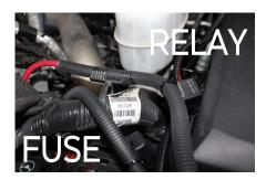
**E.** If fuse panel is located in the cab it will be necessary to guide the single red wire from the relay through the fire wall grommet to access the fuse panel.
