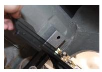
**H.** Once secure use (3)11/2 bolts and (3) WA-1001D spacers to mount the pump to the bracket.
