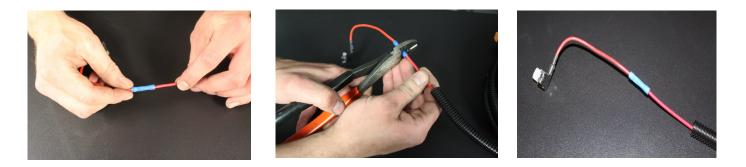
**C.** Crimp the ring terminals to the red and green wires of the WH-1006-3 Wire Harness. Attach red wire to the positive terminal of the battery and the green terminal to the negative terminal. The use of a corrosion preventative on electrical connections is recommended.
