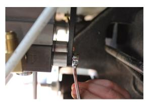
Apply motor oil to gasket located on filters. Attach to system and hand tighten. Ι.
