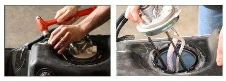
**G.** Using a cup, reach inside the tank under the hole location to catch debris. Drill a 13/8" hole. Remove debris from top of tank.
