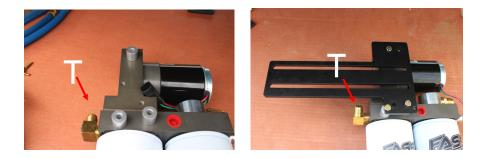
**C.** Connect female plug of the FASS harness into pump. Turn key to "on". With pump operating (you may have to bump the starter), turn pump over, liberally spray WD-40 (or equivalent) into water separator nipple lubricating Gerotor.
