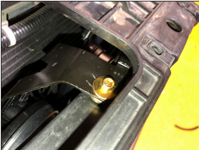
FIGURE 34 : Horn Installed w/Capture Nut, Spacer and Bolt
