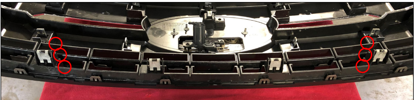
FIGURE 36 : Locations (6 Total) to Notch Factory Grille – See Close-Up Below
