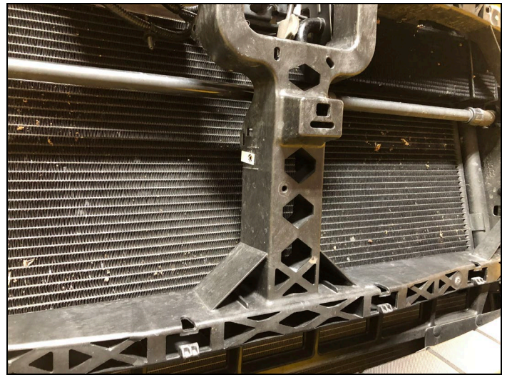
FIGURE 13 : Harness Moved and Horns Removed
