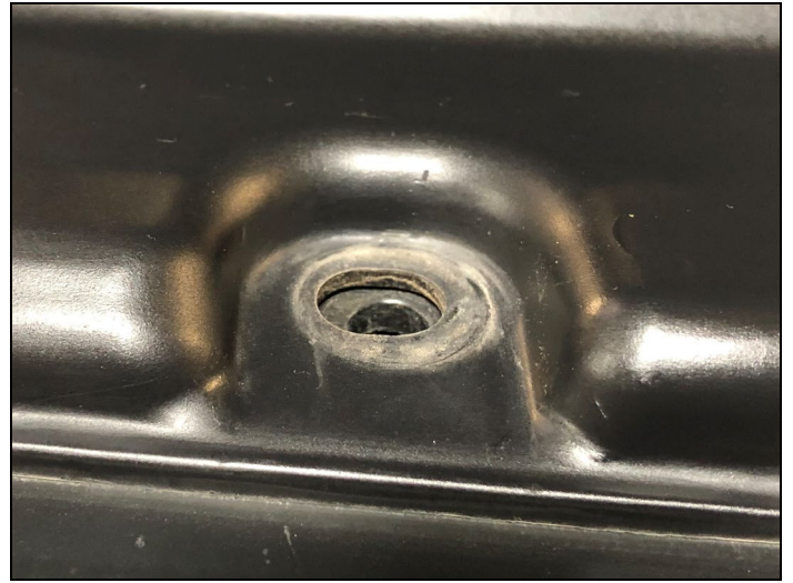
FIGURE 6 : Retainer Pin Removed
