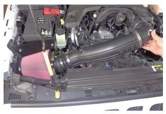
26. Install the assembled intake tube in the vehicle.
