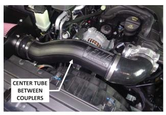
29. Center the intake tube between the couplers, then tighten the 2 remaining clamps.
