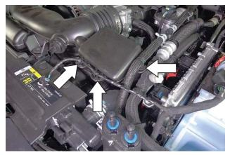
Separate the 3 wire loom clamps from the resonator.
