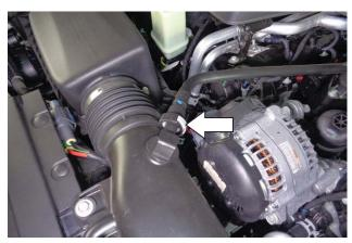
5. Disconnect the PCV line from the air inlet duct.
