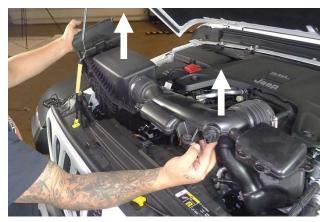
9. Pull the airbox up sharply to release it from its mount grommets, then remove the assembled airbox and ducts from the vehicle.
