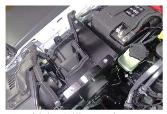
23. Install the heat shield by pressing the 2 mount pins into their rubber grommets.
