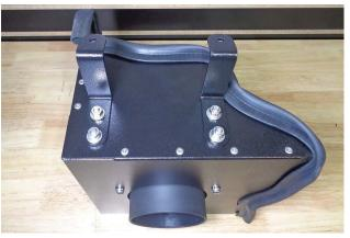
16. Attach the 2 brackets (15) to the heat shield as shown, using ½-20 screws (10) (against the heat shield), and flat washers (12), lock washers (11), and nuts (16) (against the brackets).
