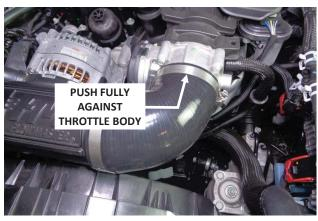
28. Push the elbow coupler up against the throttle body stops, then tighten the throttle body clamp.
