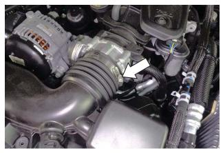
8. Loosen the screw clamp connecting the inlet air duct to the throttle body, then separate the duct from the throttle body.
