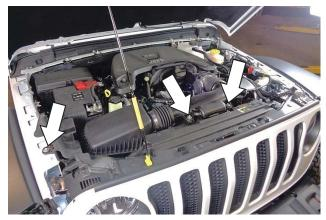
4. Remove the 3 intake mount bolts.
