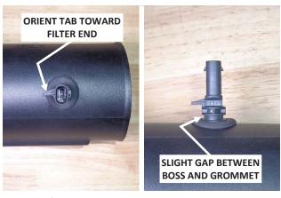
19. Carefully push the air temp sensor into the grommet, orienting the tab toward the tube's filter end. Moistening the grommet I.D. with soapy water will ease insertion. **NOTE: The sensor boss does not sit flush against the grommet; there will be a slight gap.**
