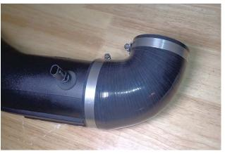
22. Slip the other #56 screw clamp (19) onto the large end of the elbow coupler (23), and install the coupler on the discharge end of the intake tube. Then slip the #52 screw clamp (24) onto the other end of the coupler. Do not tighten the clamps at this time.
