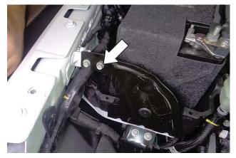
12. At the bracket just forward of the battery, remove the inboard screw.
