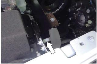
24. Secure the corner of the heat shield to the vehicle frame using the long M6 screw (9), lock washer (8), flat washer (7) and spacer (6).
