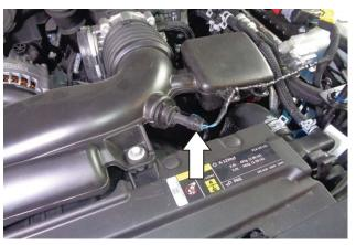
6. Disconnect the air temperature sensor plug by depressing the locking tab, then pulling it straight off the sensor.
