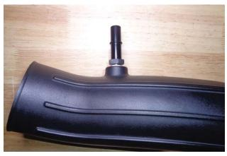
20. Apply 2 wraps of nylon thread tape to the threads of the quick connect fitting (20), and install it in the intake tube.
