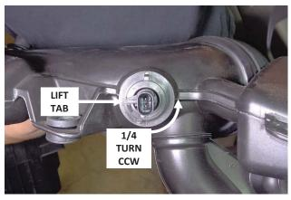
10. Remove the air temp sensor by lifting the locking tab and turning the sensor a quarter-turn counter-clockwise, then pulling it straight out of the duct. Then remove the o-ring from the sensor. CAUTION: The sensor is delicate! Handle it with care, and store it in a safe location until reinstallation.
