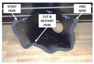
13. Attach gasket (25) to the heat shield (4), in 2 sections as shown. Firmly press the gasket onto the edge, and cut it to length using metal-cutting shears.
