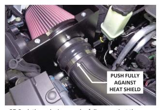
27. Push the reducing coupler fully up against the heat shield, then tighten the heat shield clamp.
