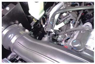
30. Connect the PCV line to the quick connect fitting and check for security.
