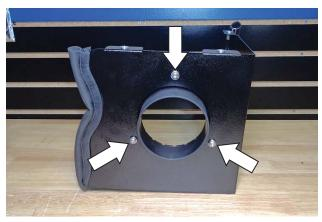
15. Assemble the air filter adapter (3) to the heat shield using M6 screws (13), lock washers (8) and flat washers (7).
