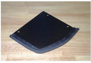
14. Attach gasket to the heat shield cover (5).
