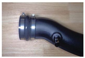
21. Slip a #56 screw clamp (19) onto the small end of the reducing coupler (18), and install the coupler on the filter end of the intake tube. Then slip the #64 screw clamp (17) onto the other end of the coupler. Do not tighten the clamps at this time.
