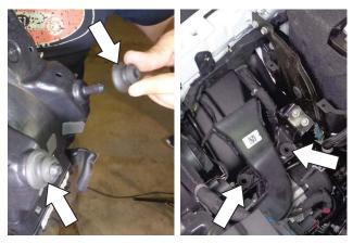
11. If either of the rubber mount grommets came out of the vehicle with the airbox, remove them from the airbox and install them in their holes in the vehicle frame.
