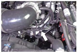
32. Use 1 or 2 cable ties (27) (as necessary) to secure the temp sensor lead to nearby wiring or plumbing.
