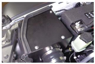
33. Attach the head shield cover to the heat shield using ¼-20 screws (10), lock washers (11), and flat washers (12).
