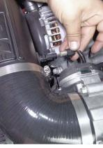
31. Connect the air temp sensor extension lead (26) to the vehicle's temp sensor plug. Then route the lead under the coupler, connect the other end to the air temp sensor, and check for secure connections at both ends.
