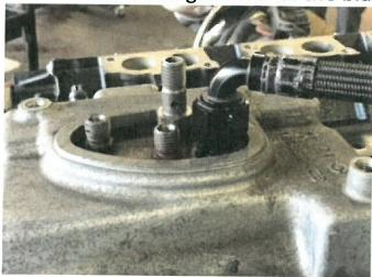
3. Install the fitting in the regulator as shown below.
