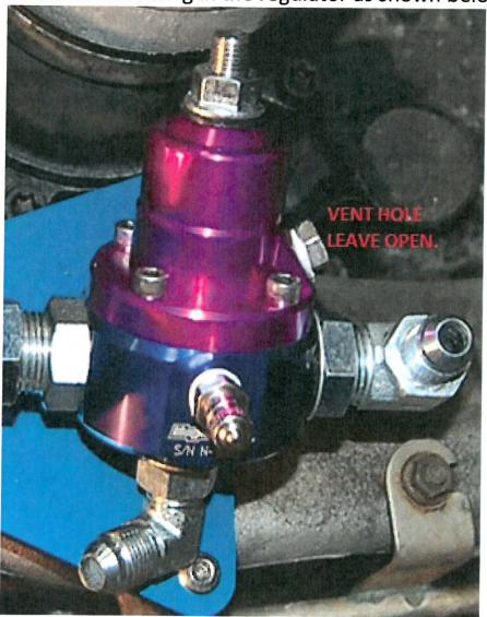
The 1/8" NPT hole in the back of the purple top of the regulator is a vent.
