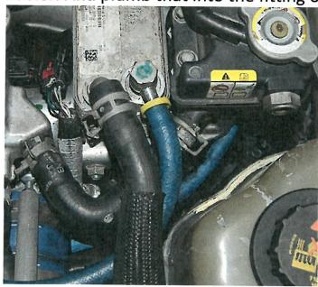
7. Once you have all the lines hooked up and tight you can set the pressure and check for leaks. Use the Schrader valve and a fuel pressure gauge to set the pressure. Desired pressure is 8-12 psi.
