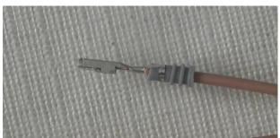
That connector has only one open hole. Two of the holes already have orange wires and two have white plugs. Plug the pin that looks like the above picture into the remaining hole. The side facing down in the picture must face the outside of the connector. If you face it the wrong way or don't slide the blue lock out of the way, the pin will not go in. The pin will go in easily. If it doesn't, something is wrong. IMPORTANT: do not use force or you might break it!
