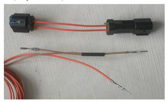
In this picture you can see the three pins on the end of the cable and the separate piece with the two connectors you need. The pins are aligned with the connectors they will plug into.
