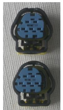
This picture shows the front of the small connector. The blue piece slides sideways as shown in the picture to the left. To plug it into the truck, it must be centered like the top connector in the picture. In order to insert the pin, it must be slid to the side (as shown in the lower connector in the picture).
