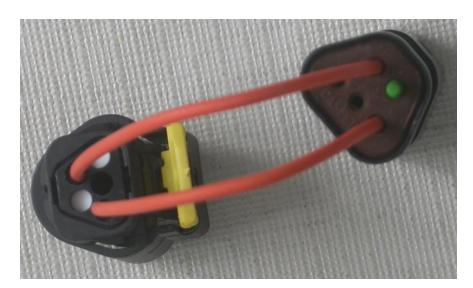
In this picture you can see the three available holes into which you will plug the three pins. Do not plug anything into the holes with the white or green plugs and make sure to leave them in place. They are there to keep water from entering the connectors. Make sure your cable looks exactly like this picture.
