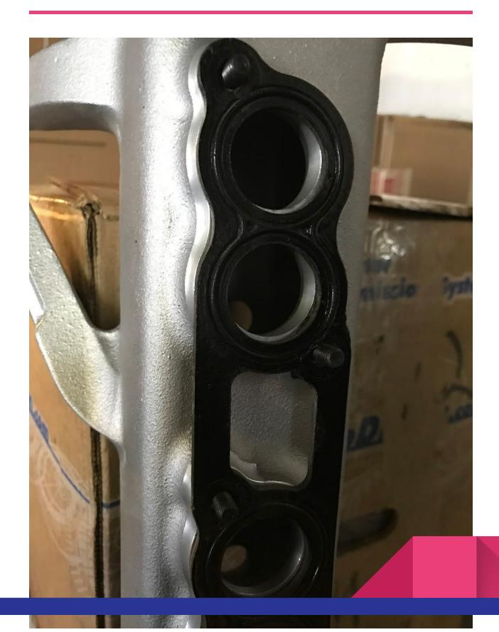
Lay the manifold on top of the motor. Begin tightening the bolts by hand. (We use a 5mm 4in Allen socket for a ¾ drive ratchet). Once the bolts are all started and snugged up by hand begin to torque them to 9ft pounds. Re check torque when done. Use the factory bolts on the rear of the manifold. Once that's done begin to thread the Allen plugs by hand and tighten by hand till they stop turning. (No extra force is required).
