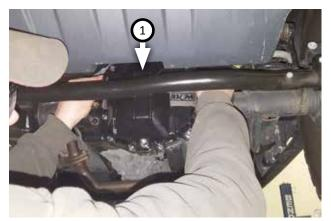
7. Place factory gasket (removed step 4) onto **front differential cover (1)**. Secure them to front differential using screws (x2) on both sides as shown.
