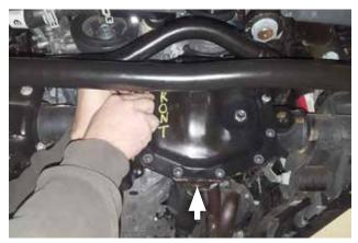
3. Place drain pan under front differential where it can catch fluid. Remove factory plug and allow fluid to drain. Then remove bolts (x12) and differential cover.
