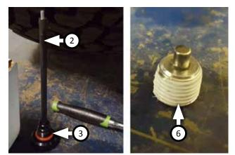
6. Install o-ring (3) onto dipstick (2). Wrap drain plug(6) with Teflon tape (about 2 wraps).
