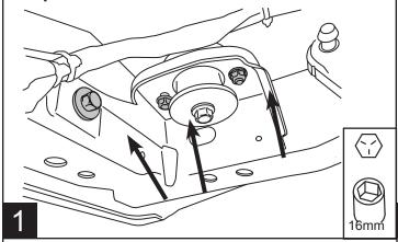
Using a 15mm wrench assemble steel bracket to
