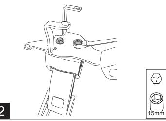
Drop threaded plate into slot in frame. Slot is located on both sides of the frame. The outer slot is preferred but may not be accessible with aftermarket bumpers or racks.
