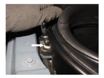
Install the Step Coupler (M) onto the throttle body with the Hose Clamps #48 and #52 (N & L). Tighten hose clamp #48.
