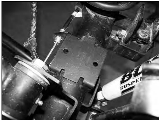
12. Install brakeline relocation brackets to the original brake line mounting point on the frame. Attach the bracket with the factory bolt. Attach the brake line to the INSIDE surface of the drop bracket with a 1/4" x 3/4" bolt, nut and washers (Fig 7). Torque hardware to 10 ft-lbs.
