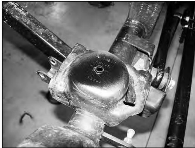
10. Place a provided bump stop spacer (3296) inside one of the springs. Install the spring in the vehicle with new spring spacer on the top of the spring. Make sure the spring is seated properly in the axle mount. The OE upper spring isolator should be reinstalled with the spacer to net the full 2" of lift.
