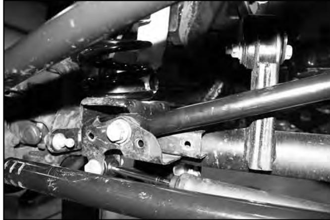
4. Raise the front of the vehicle and support the frame with jack stands behind the front lower control arm pockets.
