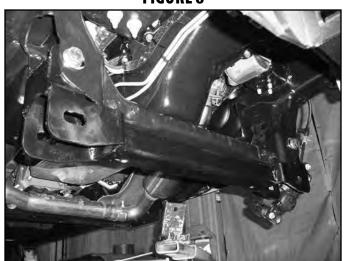
19. Install the front crossmember in the front lower control arm pockets and fasten with the OE lower control arm hardware. Run bolts from front to rear (Fig. 9). Leave hardware loose.
