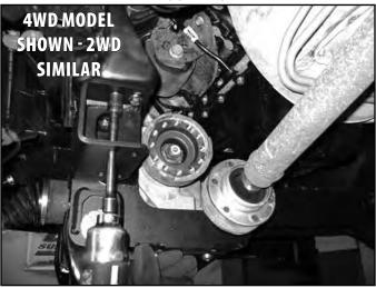
23. With the lower control arms installed, go back and torque the four crossmember mounting bolts to 222 ft-lbs. Ensure that the front crossmember is centered in the vehicle. Apply Loctite to the threads and torque the crossmember support bolts to 50 ft-lbs. Tighten sway bar drop hardware to 35 ft-lbs.
