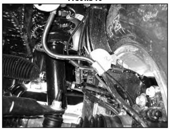
37. Install the sway bar to the new sway bar drop brackets (Fig 17) with 7/16" x 1-1/4" bolts, nuts and washers (BP 407). Attach the sway bar to the sway bar end links with the original hardware. Torque the 7/16" hardware to 45 ft-lbs. Torque sway bar link nut to 45 ft-lbs.
