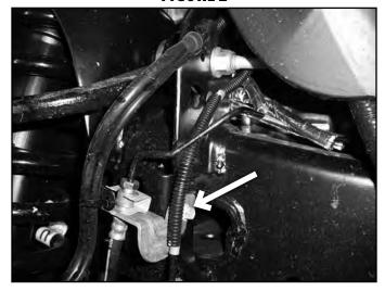
7. Disconnect the tie rod ends from the steering knuckles. Remove and retain the mounting nuts. Avoid hitting the aluminum steering knuckle, use appropriate tool to remove tie rod end from steering knuckle. Take care not to strike the tie rod end, or damage the threads. (Fig 3)
