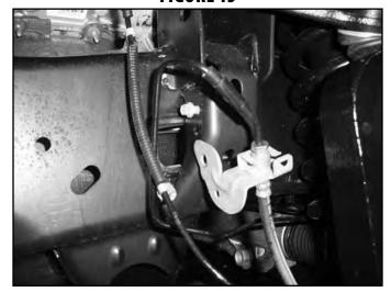
36. Attach the ABS line to the connector at the inner fender. Route the lines similar to the factory setup down to the side of the knuckle. Attach the ABS wire with the factory 6mm bolt to the side of the knuckle. Attach the brake line with a new 6mm x 18mm bolt with 1/4" washer to the side of the knuckle (BP# 773), the brake line locating tab will go into the unthreaded hole. (Fig 16).
