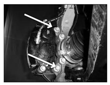
6. Disconnect the ABS lines from the retaining clips. Disconnect the brake line bracket from the frame rail. Disconnect the ABS line from the hub assembly. (Fig 2).
