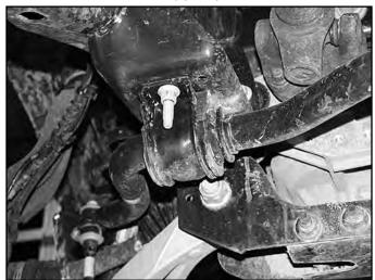
12. Loosen but do not remove the three strut assembly mounting nuts at the frame (Fig 6). Do not loosen the middle strut nut.
