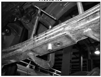
52. Install the new provided lift block so that the bump stop wing goes toward the inside of the vehicle. The block will use the both of the lower center pin holes. The upper only uses 1 hole which will shift the axle slightly forward.
