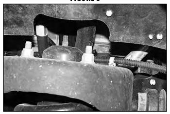
13. Remove the strut-to-lower control arm hardware. Save bolt and nut.
