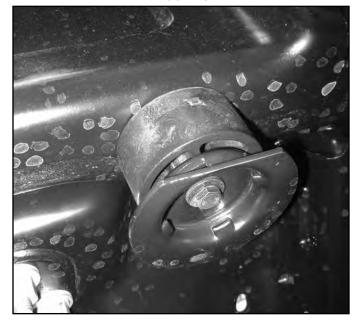
18. Grease the bump stops and reinstall into the factory cups. Raise the axle to get the bump stops to press into the cups. (Fig 10)
