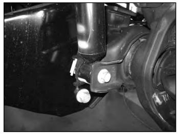
11. Disconnect sway bar from the frame. Retain (4) mounting nuts. (Fig 6)
