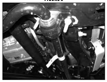
12. Lower the axle and remove the factory coil springs.
