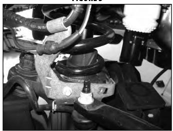
9. Disconnect the brake line bracket frame (Fig 4). Retain hardware.
