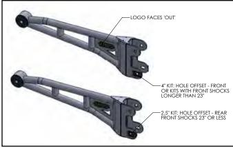
15. Tighten the radius arm hardware at the axle to 222 ft-lbs. Do not tighten the pivot bushing at the frame. (Skip ahead to bump stop installation)
