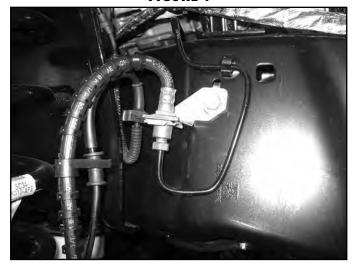
10. Disconnect the shocks by removing factory hardware (Fig 5a, 5b). Retain lower bolt and nut tab for later reinstallation.
