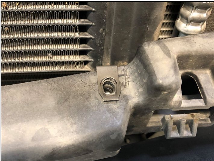
FIGURE 6 – Hole Drilled & Clip Capture Nut Installed
