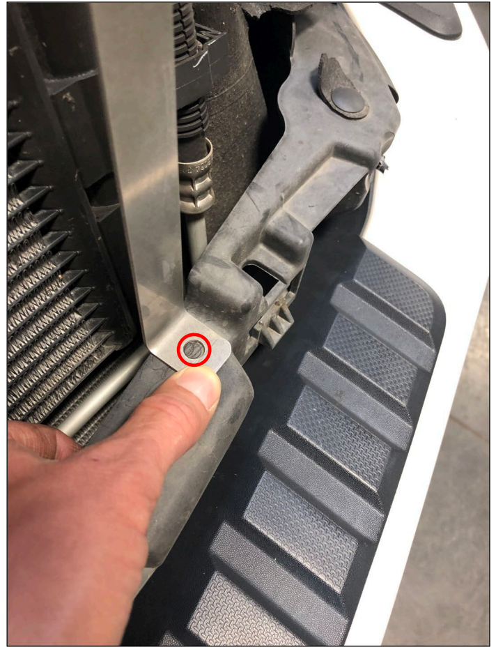
FIGURE 5 – Marking Hole Location
