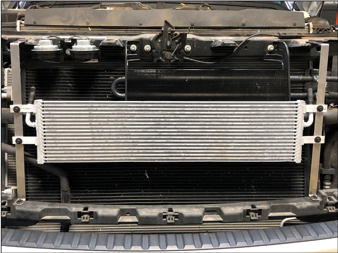
FIGURE 8 – Transmission Cooler Mounted
