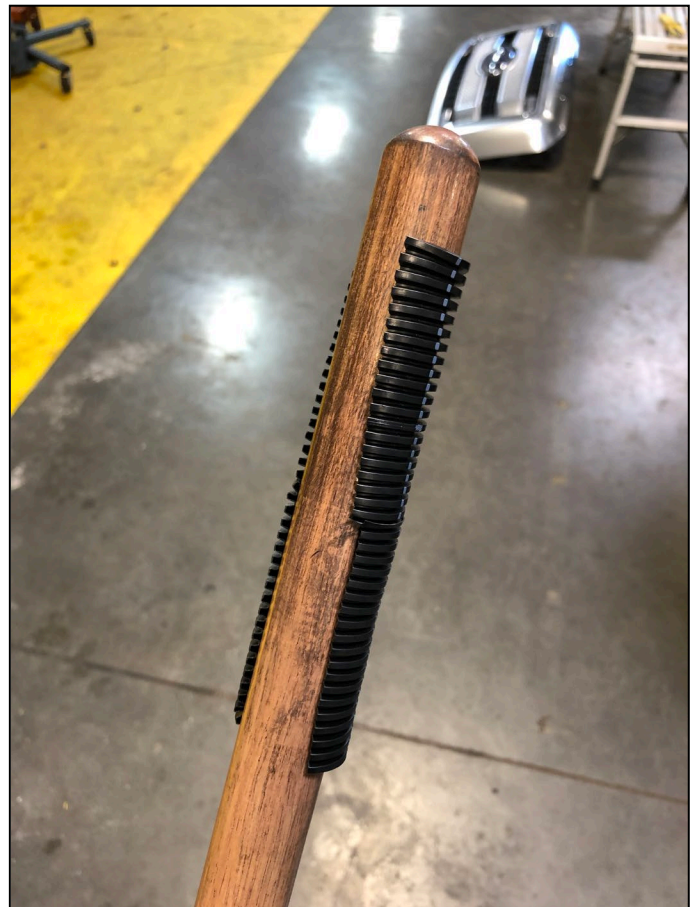
FIGURE 10 – Stretching The Loom Makes It Easier!
