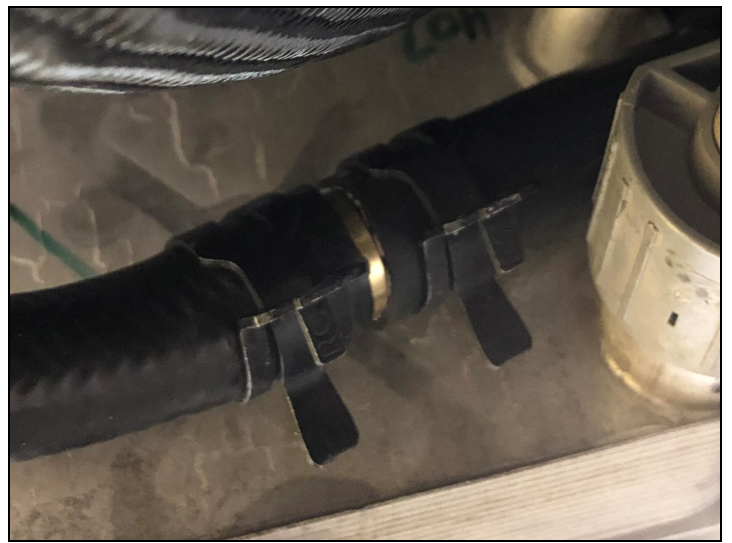
FIGURE 18 – Hose Coupler Installed with Clamps
