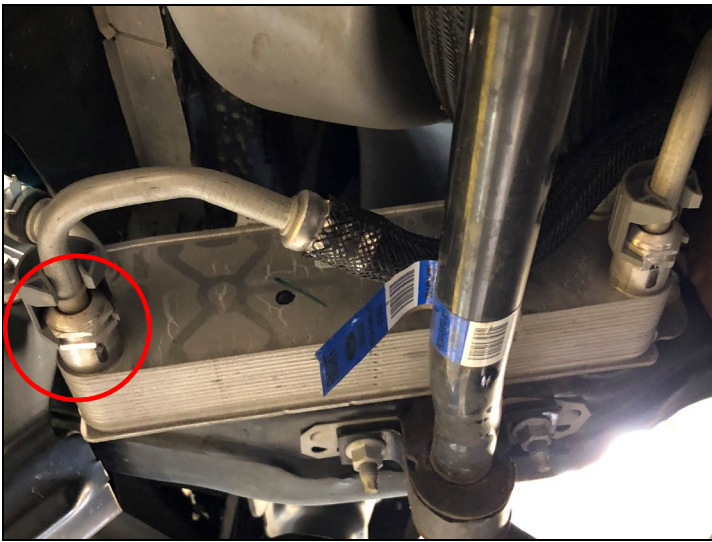
FIGURE 15 – Stock Trans Cooler – Outlet Marked
