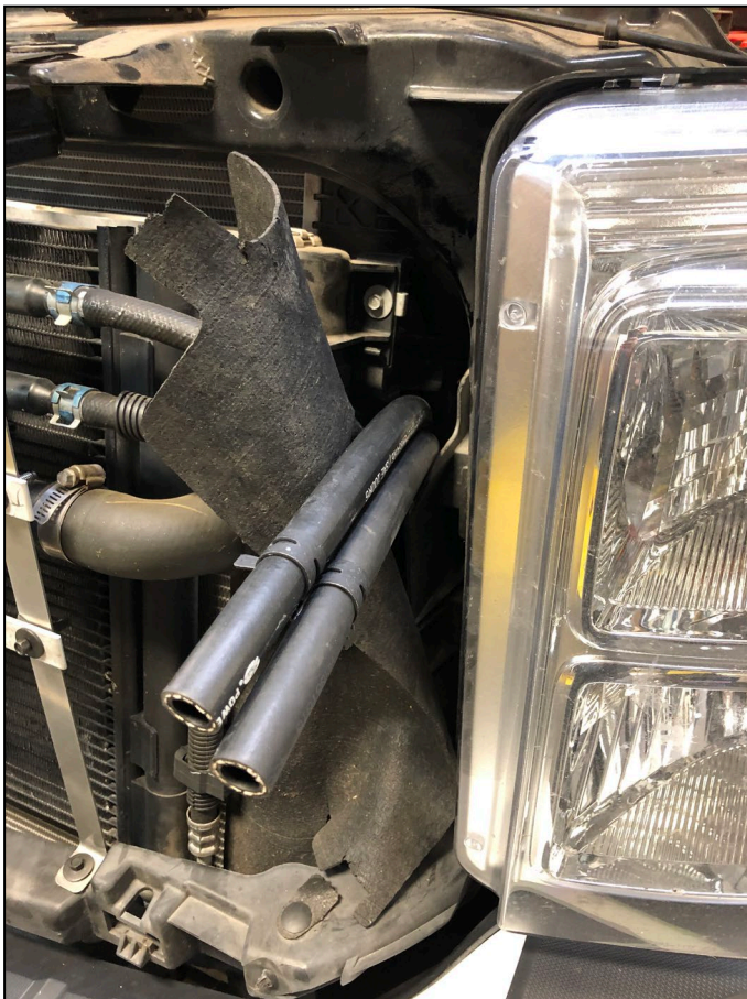
FIGURE 9 – Driver Side Hose Routing Location
