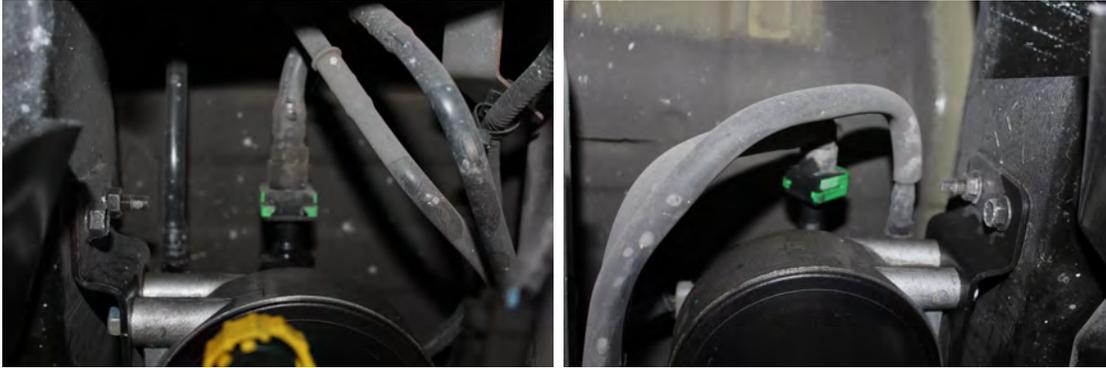
D. Remove the (4) bolts that secure the OEM fuel filter housing and remove the housing from the truck.
