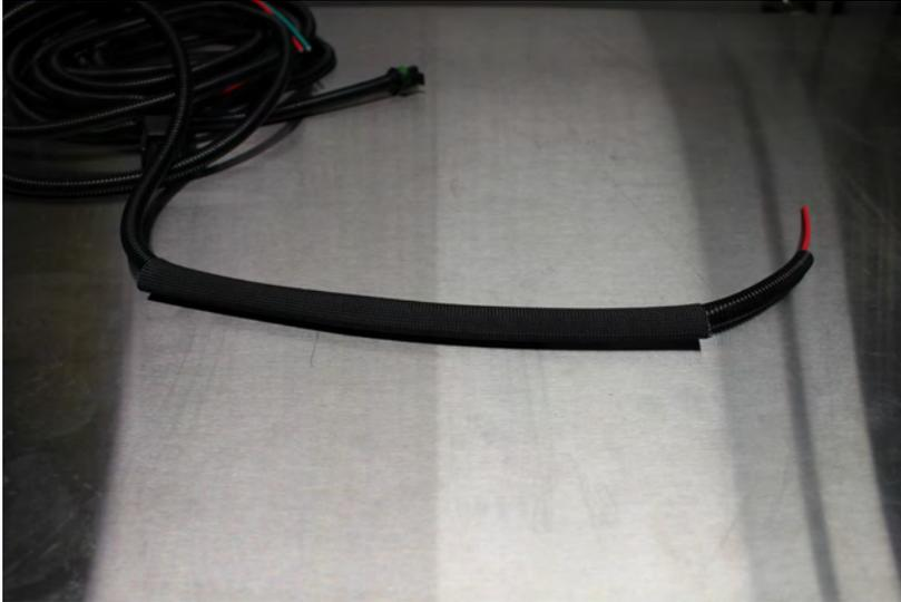
E. Route the single red wire of WH-1006-3 to the engine bay fuse panel on the passenger's side. Remove a fuse (maximum of 10A) that is "hot" when the key is on. Use a test probe to locate the "hot side" of the circuit in the fuse block. Install the Add-A-Circuit into the open location. Install the pulled fuse into the open space on the fuse tap.
