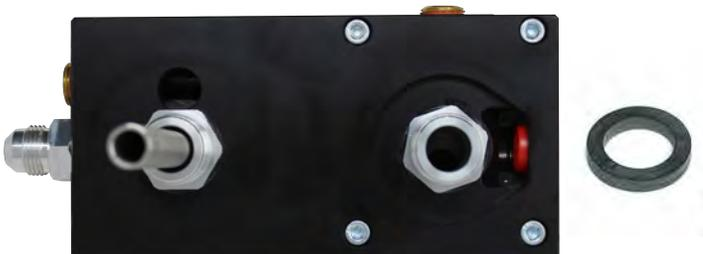
**Note: O-Ring must be put back on suction side of pump. Failure to do so can result in priming issues, cavitation or pressure losses.**
