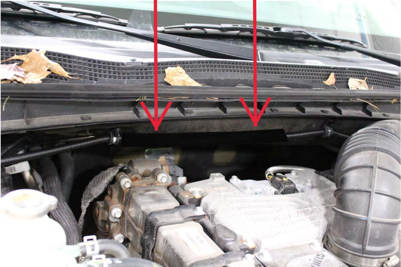
G. Route WH-1006-3 wire harness along frame rail to mounting location of pump. Completion of this step will be addressed in the mounting step.
