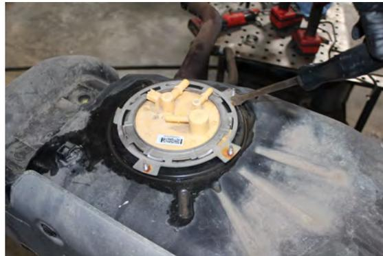
H. Disconnect the fuel level sending unit electrical connector to prevent damage to wiring, this will be reconnected prior to reinstalling the fuel tank module.
