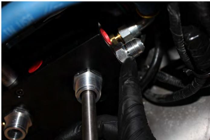
**E.** Install the remaining section of FL-1002 onto PL-2003 using oil. Install PL-2003 onto the FASS engine feed fitting 10-300, in some cases it may be necessary to remove the FASS return fitting. If removed, be careful to not damage the FASS pressure spring!
