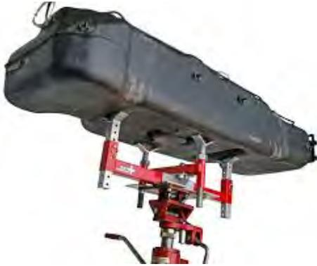
G. Remove and discard the fuel tank module shield, this will no longer be used. Clean the fuel module area then remove the lock ring on the top of the fuel tank. **This is spring loaded, so, holding it down while removing the ring will prevent the sending unit from popping up and possibly causing damage.**
