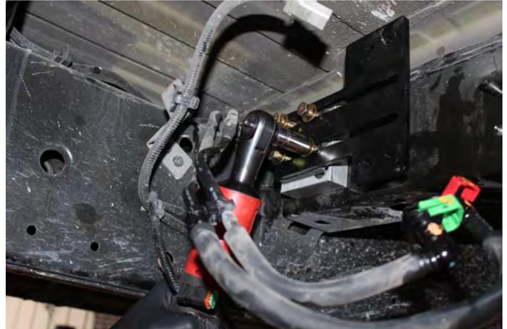
D. Install (3) 1/4" bolts with (3) WA-1001D spacers as pictured below. Tighten the (4) 3/8" bolts from step C, be sure PBR-2002 is level.
