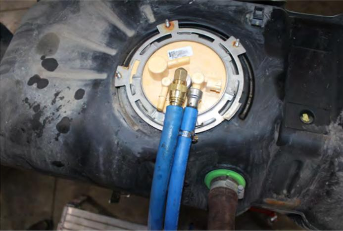
**S.** Remove and discard the OEM fuel feed line from the truck, this will no longer be used.
