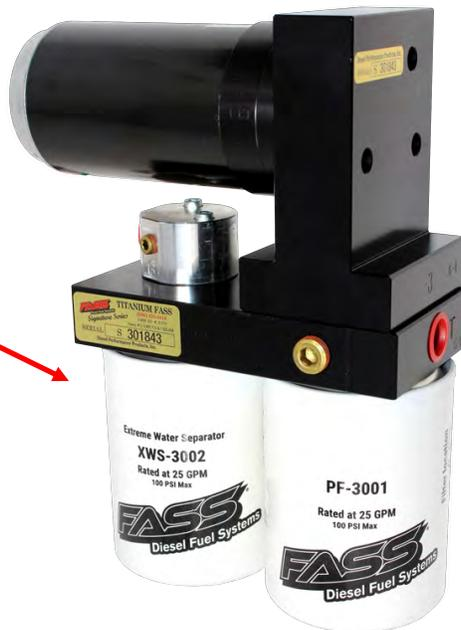
**Particulate Filter - Install PF-3001 on filter nipple without the draw tube. Make sure to insert O-Ring provided on nipple.**
