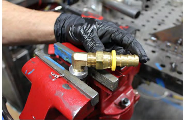
L. Install QD-1002 onto the OEM suction line on the fuel tank module.
