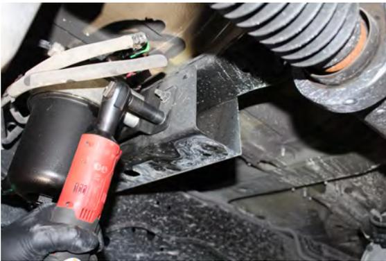
E. Remove the fuel tank skid plate, disconnect the fuel fill and vent tubes.
