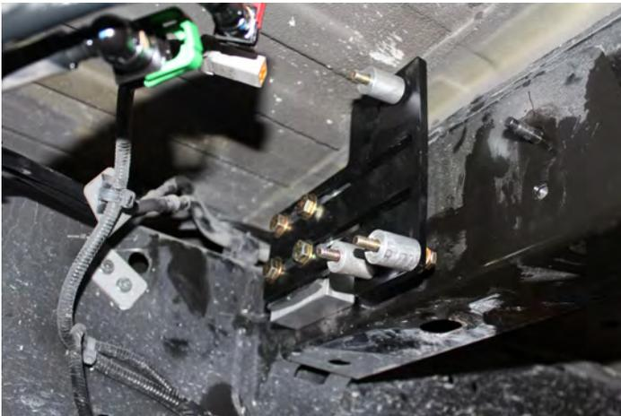
E. Install the FASS onto the (3) 1/4" mounting bolts and tighten accordingly.
