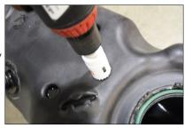
K. **VERY IMPORTANT:** Support fuel tank on both ends allowing the natural formation of the tank to take place. Failure to perform this step can and will create an issue with less usable fuel!
