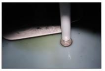
M. With proper length being obtained, place the assembly into the drilled hole securing the assembly using the lock washer & nut. Tighten Nut. Loctite may be applied to the threads of the BHF-1002 for added insur-
