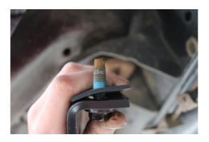
B. Secure THB-1001 to bolt on bracket with the RS 1002 and the (2)–1/4-20x1 bolts, 1/4 washers, and 1/4 nuts. With the (4)-1/4-20x1.75" bolts thread the BHB-1001 to the THB-1001.
