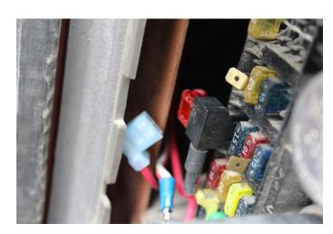
G. Route WH-1005 wire harness along frame rail to mounting location of pump. Completion of this step will be addressed in the Mounting Step 3.
