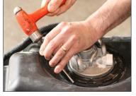
G. Once the lock ring is removed, remove pick up module from fuel tank. Be careful not to bend the fuel sending arm.
