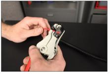
B. Place wire from 46044 and WH-1005 into butt connector. Using crimping tool connect 46044 and WH-1005 with butt connector. Install 46260 to 46044 bottom slot (opening that is near the spade). Route Add-a-fuse lead through the fire wall using existing grommet. The use of corrosion preventative spray is recommended.
