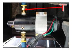
B. Install in-line fuel filter in an accessible location in the suction line using the HC-1001's. Make sure the fuel flows in the direction of the arrow on the canister.
