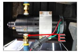
D. Measure and cut fuel line. Insert PL-2003 90° Push-Lok fitting using oil.
