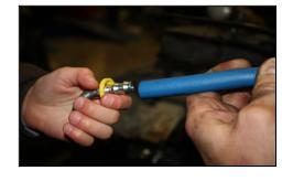
E. Disconnect factory fuel line and injector return line from inlet side of the factory fuel filter and install the DIPF-1003. Torque to 18 ft./lbs.
