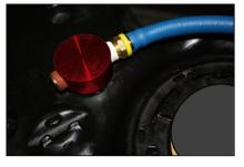
O. Carefully reinstall install pick up module making sure the leveling arm is not obstructed by the suction tube. Reinstall factory lock ring. Push one end of fuel line onto 'S' port of suction tube assy. Loop fuel line over frame. Do not cut at this time. Reinstall fuel tank making sure to reconnect factory suction, return, electrical connections, and filler neck tubes. Torque hanger bolts to factory specifications.
