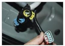
C. Disconnect factory suction and return lines. Refer to diagram at the beginning of Step 2
