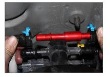
H. Clean and cap off the factory return ports with the two RVC-38 caps. Clean and cap off the factory feed port with the RVC-12 cap. Seal factory electrical connection with di-electric grease or similar to prevent corrosion.
