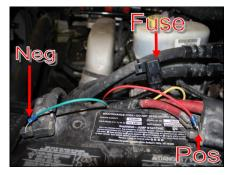
D. Secure relay and fuse in an upright position, as shown, to prevent moisture from entering. Di-electric grease may be applied to prevent corrosion.
