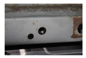
B. Secure PFB-2002 and RS-2001 with (1) hex bolt 1/2" -20 x 1 1/2" and (1) 1/2" washer to FPB-2005
