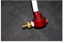
J. Place the lock ring back on the tank and locate the BHF-1002 bulkhead fitting on the tank with enough clearance for the fuel line and fittings. **Keep in mind the bulkhead must also clear the bottom of the bed support structure.** The fiberglass protective shell will have to be trimmed as necessary for clear-
