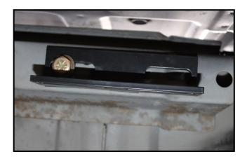
C. Secure THB-1001 to bolt on bracket with the RS-1002 and the (5)-1/4-20x1 bolts, 1/4 washers, and 1/4 nuts. With the (4)-1/4-20x 1.75" bolts thread the BHB-10001 to the THB-1001.
