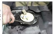
E. Clean the fuel module area then remove the lock ring on the top of the fuel tank. This is spring loaded, so, holding it down while removing the ring will prevent the sending unit from popping up and possibly causing damage.
