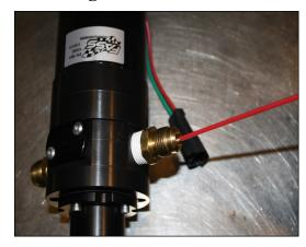
E. Slid the FASS pump into mounting brackets with the weep hole facing down. Torque (4) bolts to 110 inch pounds.
