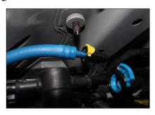
G. Disconnect both factory return lines from the factory lift pump (Refer to diagram at the beginning of Step 2). Insert DB-4646 into each return line fitting until you hear a click and tabs lock.
