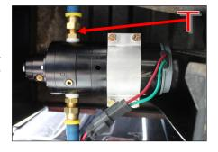
B. Install in-line fuel filter in an accessible location in the suction line using the HC-1001's. Make sure the arrow is in the direction of the fuel flow.
