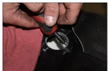
M. Place the bulk head assembly into the drilled hole, take measurements so the bottom of the suction tube is only 1/8" (no more than 2 quarters stacked) from the bottom of the fuel tank. **Measure twice and cut once!** Using a razor knife, cut to proper length. If unsure of correct length, make small cuts until proper length is achieved.
