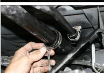
Helpful Hints: If more space is required to access the top of the fuel tank, loosen the strap nuts to the end of the stud. This will gain you about 3" more working room.
