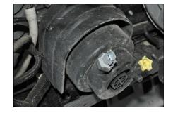
E. Disconnect the yellow-clipped factory feed at the factory lift pump. Refer to diagram at the beginning of Step 2.
