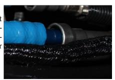
H. Measure between the two factory return fittings. Insert two PLB-1238 fittings into the provided FL-1002 fuel line using oil. Insert fuel line into factory quick disconnects until you hear a click. Lock down retainer clip. Secure fuel line and wire harnesses.
