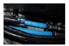
Note: Secure all fuel lines with cable ties. Cable ties are an economical way to prevent the possibility of problems occurring!
