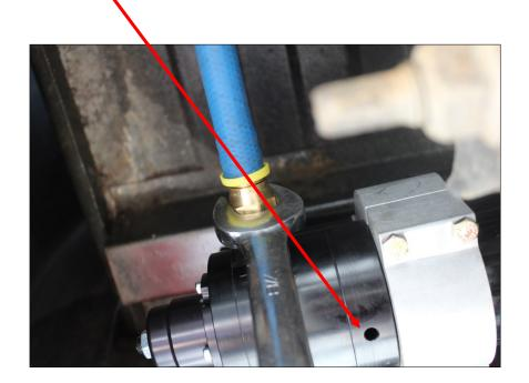
F. Disconnect the factory power plug to the HFCM lift pump. Clean plug and install the WE-1006 extension connector. Plug female plug of the WH-1002 harness into pump. Reconnect the battery. Turn key on. With pump operating, liberally spray WD-40 (or equivalent) into the "T" port. This process helps lubricate the gear for easier initial priming.
