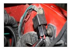
C. Route wire harness along frame to the approximate mounting location near the fuel tank. **Completion of this step will be addressed in the Step 3.**
