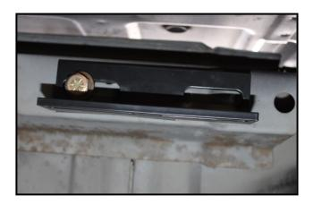
C. Secure THB-1001 to bolt on bracket with the RS-1002 and the (5)-1/4-20x1 bolts, 1/4 washers, and 1/4 nuts. With the (4)-1/4-20x 1.75" bolts thread the BHB-10001 to the THB-1001.
