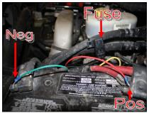
B. Secure Relay in an upright position, as shown, to prevent moisture from entering. Di-electric grease may be applied to prevent corrosion. Examples of locations to secure relay:
