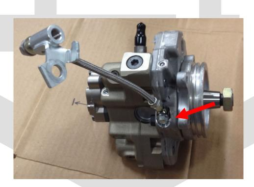
Pump has a feed line for the HCI dosing system attached to side. DO NOT loosen this line on the pump (red arrow)
