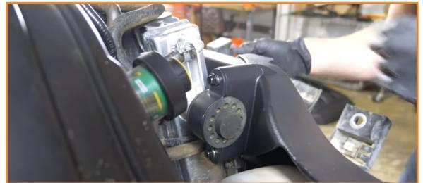
12. Reinstall the hood sensor bracket. (1x 10mm bolts, 1x washer, 1x lock washer)
