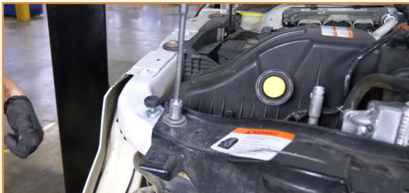
7. Separate the electrical connector from the support bar and remove the hood sensor bracket. (1x 10mm Bolt)
