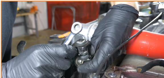
8. Remove the bolts and brackets that secure the radiator. (4x 10mm bolts)
