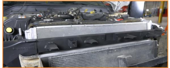
11. Secure the radiator using the radiator support brackets from your kit. (4x 10mm bolts, 4x washers, 4x lock washers)
