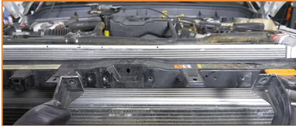
6. Remove the bolts that secure the upper support bar to the front end. (6x 13mm bolts)
