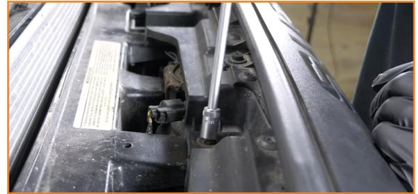
2. Remove the clips on the grille on both the driver and passenger side. (2x pop-clips)
