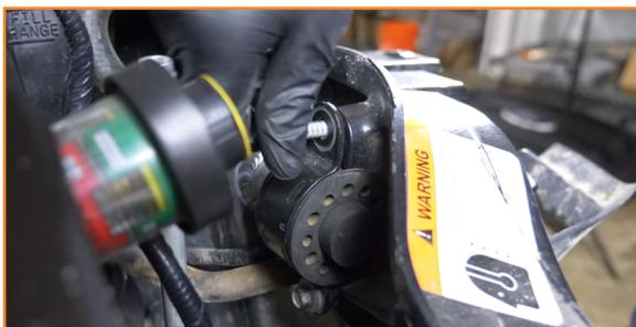
9. Free the radiator by removing the two radiator supports. (2x 10mm bolts)
