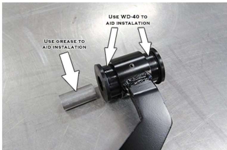
Figure 1: bushing and crush sleeve installation
