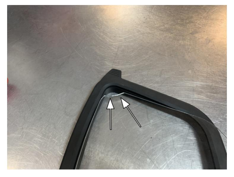
Install the Silicone Snap-in Lid seal (B) onto the S&B Clear Lid (A). Line up the lid notch feature on the lid into the silicone part underneath the pull tab so it is oriented in the seal properly. Continue to pull the seal over the edges of the lid until the lid is securely completely within the silicone snap-in seal. the mating feature on the silicone part is underneath the pull tab.
