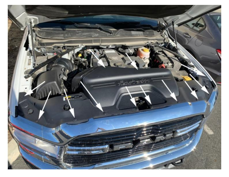
Remove the panel push-in rivets attaching the air scoop cover. There are 12 in total. Be sure to remove the two in the rear of the scoop cover connected to the factory scoop. A step stool may be required to reach.
