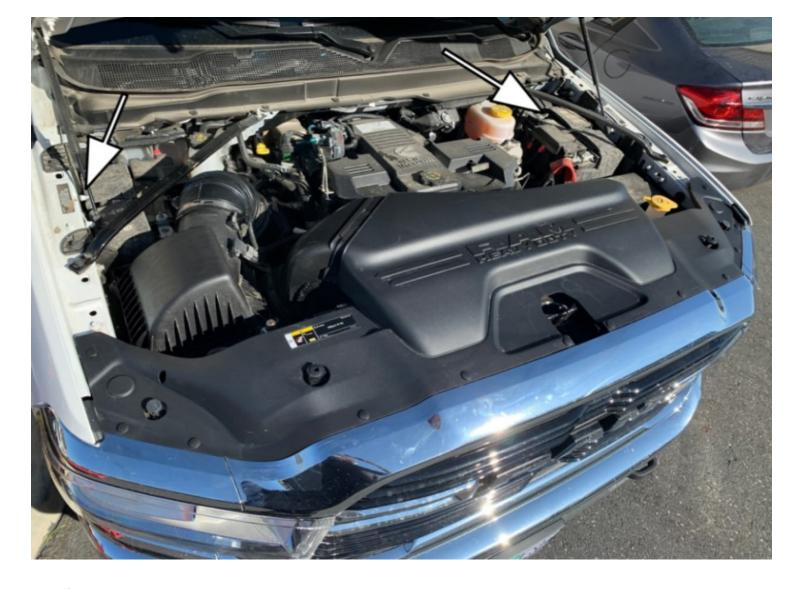
With the ignition switched off and the parking brake set, open the hood and disconnect the negative battery cable on the drivers and passengers side of the engine.
