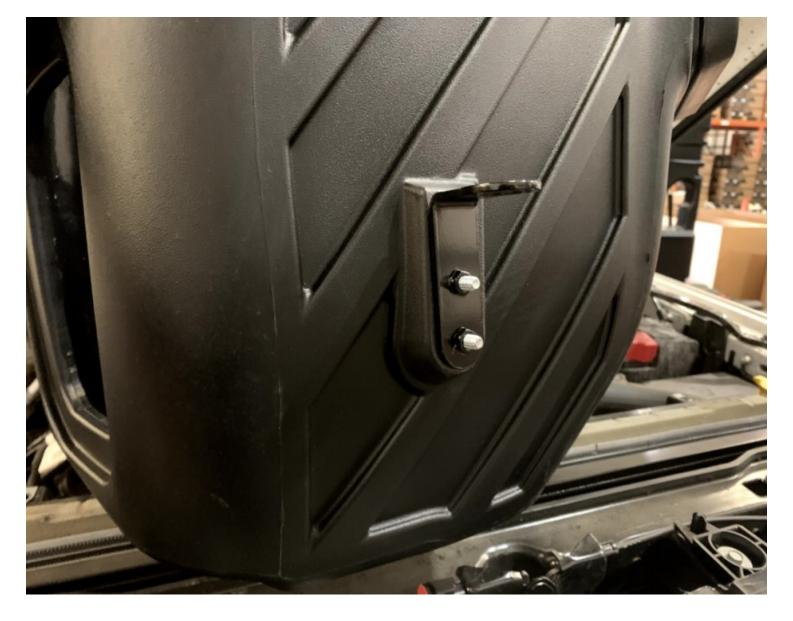
Attach the mounting bracket (G) to S&B airbox (J) by securing the  $\frac{1}{4}$ "-20 screws (D) and  $\frac{1}{4}$ " washers (E) using an 11mm socket or driver.
