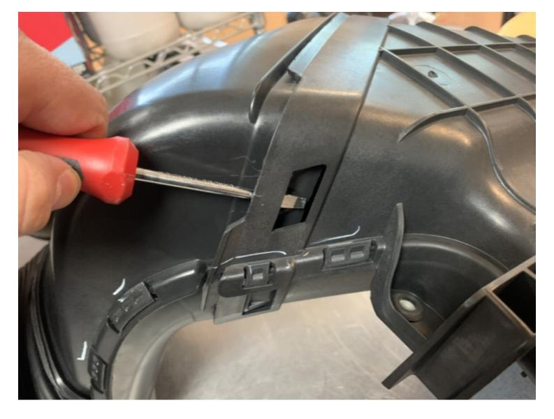
Remove the top portion of the scoop by prying the tabs to the sides of the scoop from the factory intake assembly using a flathead screwdriver.
