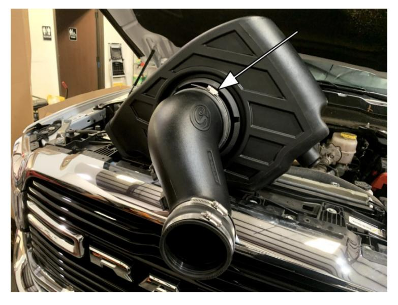
Attach the tube (C) to the filter flange and slightly tighten the #104 hose clamp (I) using a 5/16" driver or socket. Allow the tube to be able to rotate for later in the installation
