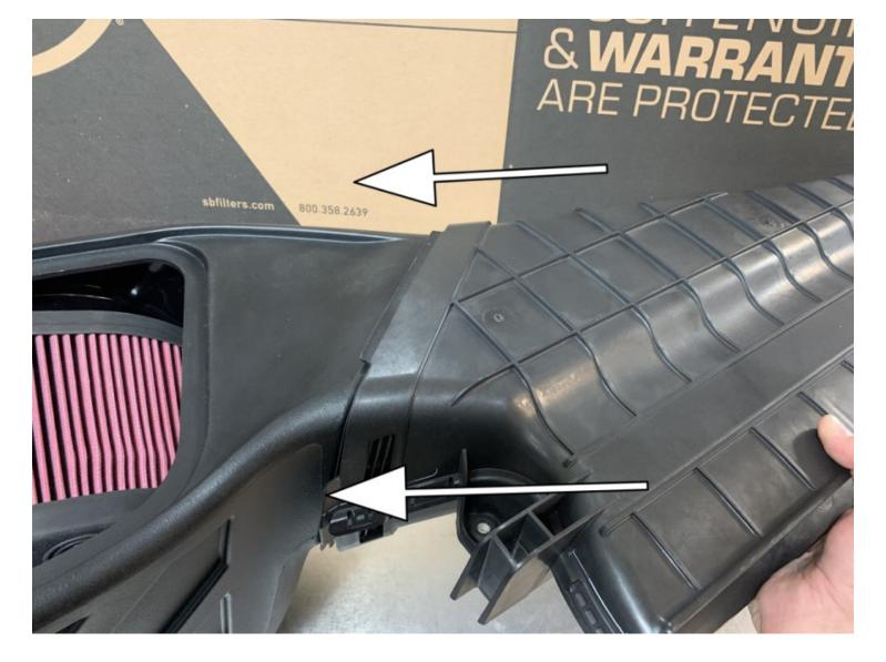
Align the factory scoop with the S&B Airbox (J). Push the factory scoop over the S&B scoop seal (V).
