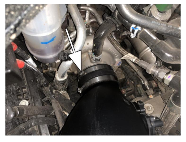
Line up the #64 hose clamp (U) over the turbo body and push on the coupler at the turbo. Tighten the hose clamp using a 5/16" driver or socket (possible socket extension).
