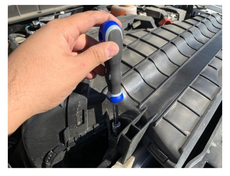
Remove the 2 bolts attaching the factory air scoop to the vehicle using a 10mm driver or socket. Collect these bolts and set them to the side, to be re-installed later.
