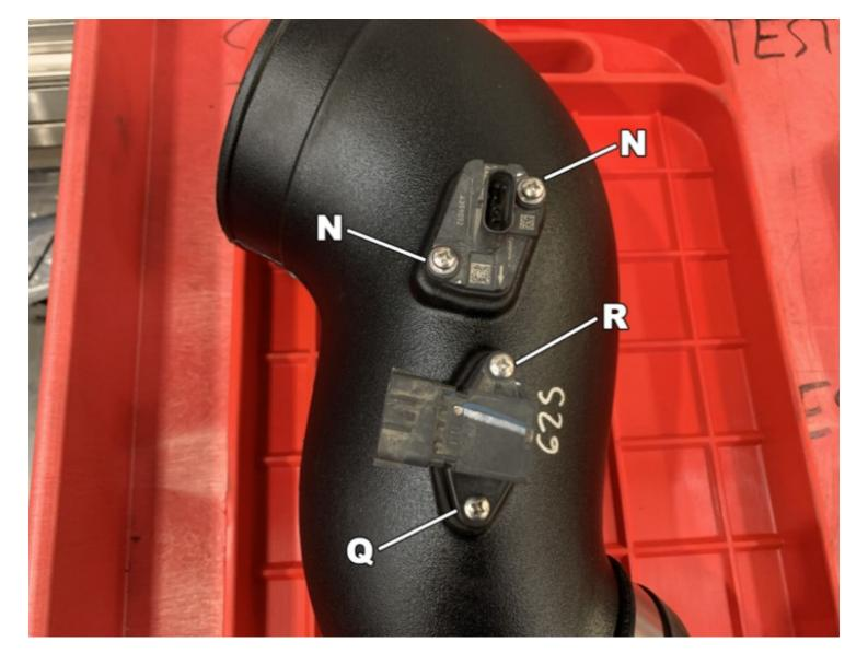
Assemble onto the S&B Tube (K) the gaskets and sensor pads for the IAT and MAF (O, L, P & M). Secure the sensors with the #8-32 pan head screws provided (Q & R & N) using a Phillips screwdriver.
