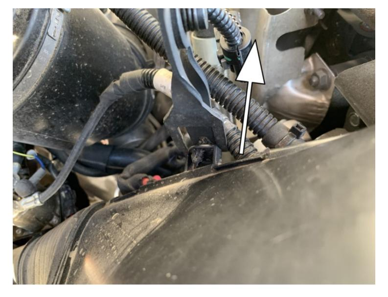
Using a panel popper remove the panel rivets securing the electrical harness connected to the factory air box and air scoop locations
