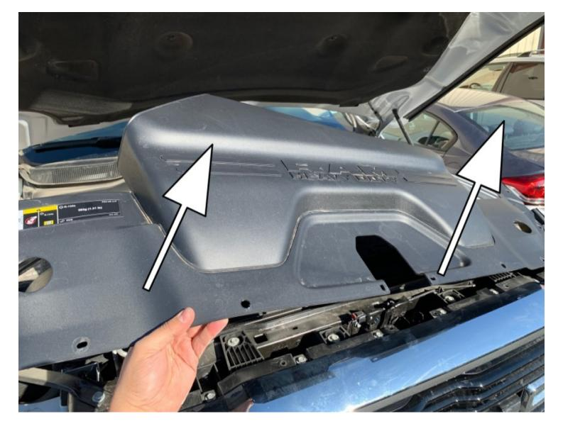
Lift-up the factory air scoop cover and remove it from the vehicle. Set it to the side, to be re-installed later
