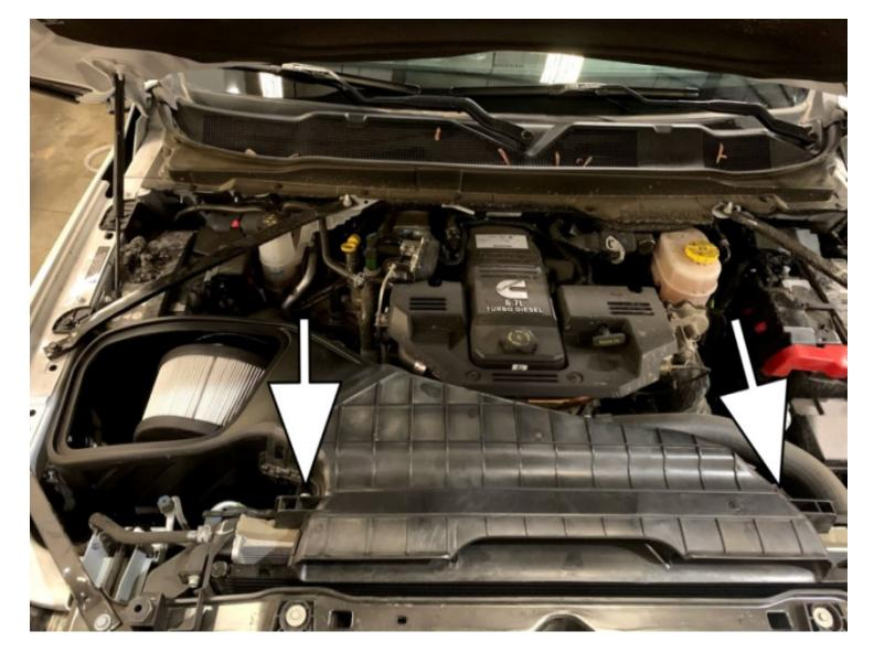
Lineup factory scoop into the factory position and tighten the bolts, removed in step 4, using a 10mm socket or driver.
