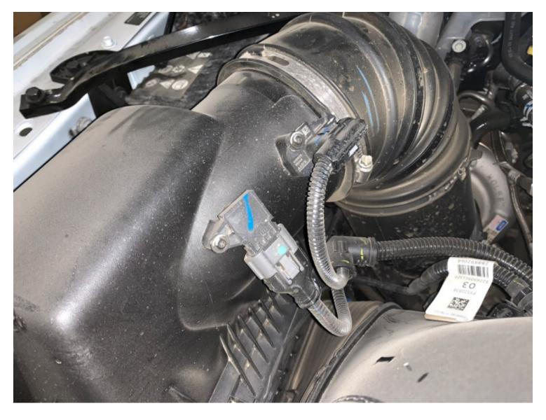
Disconnect the Intake Air Temp (IAT) and Mass Air Flow (MAF) Sensors from the stock airbox.
