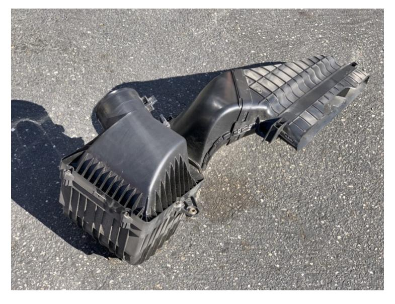
Firmly Lift up and remove the entire factory intake assembly from the grommets of the vehicle. Set the assembly to the side
