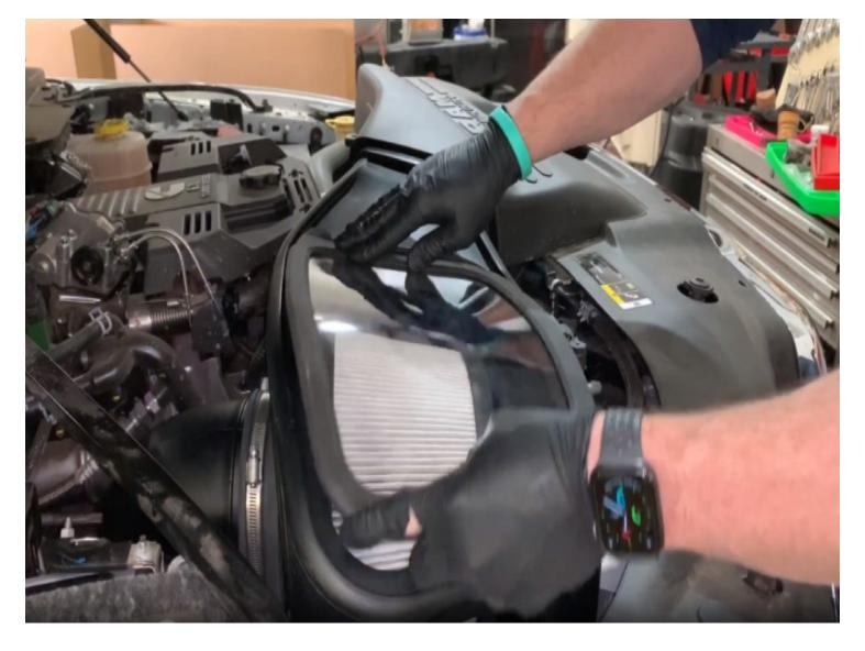
Install the S&B Snap-in Clear Lid onto the S&B Air box by inserting one corner or edge of the seal fully first, then work around the lid by pressing on until each section has snapped in
