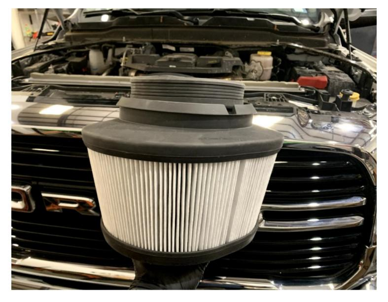
Install the Silicone S&B Snap-in Air Filter (C) onto the S&B Airbox (J)
