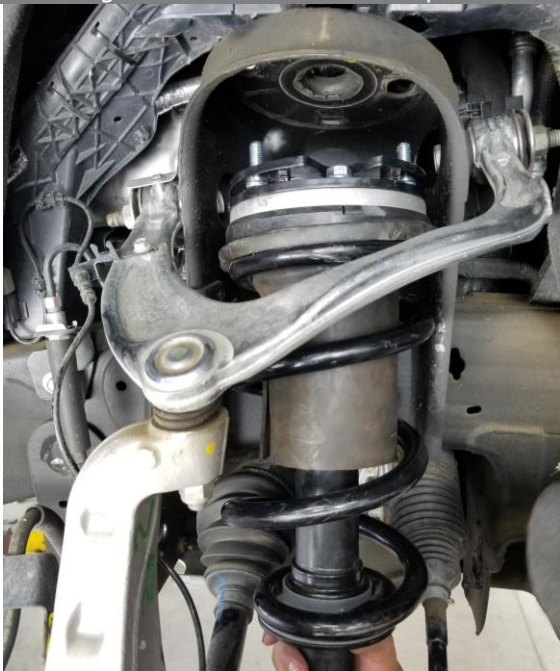
Figure 13: Install Strut With Spacer
