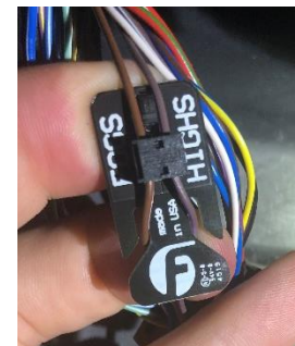
Install cover to seat wires
