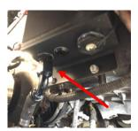
STEP 5: Install the cap and overpressure bleed hose.
