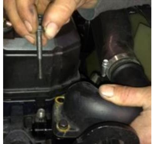
STEP 7: To allow for clearance to the freeze plug at the rear of the engine block, remove the "L" shaped bracket located between the engine and top of the transmission. Remove the large 58mm (2 ¼") freeze plug at the rear of the engine block. From underneath the truck, using a 36" pry bar and hammer, drive the outer edge of the freeze plug in to rotate it in its bore. Remove the freeze plug from the block.
