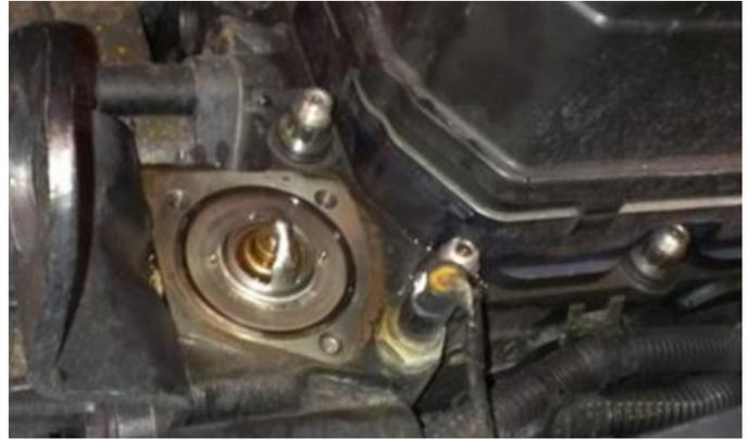
STEP 4: Remove the stock thermostat. Inspect it for wear and proper function. With a Scotch-Brite™ pad and degreasing solution, thoroughly clean the sealing surface of the stock thermostat and thermostat housing. Be sure to remove any foreign debris, and reinstall the OE thermostat.
