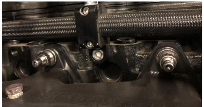
*NOTE: Ensure the coolant line does not contact the exhaust manifold.*
