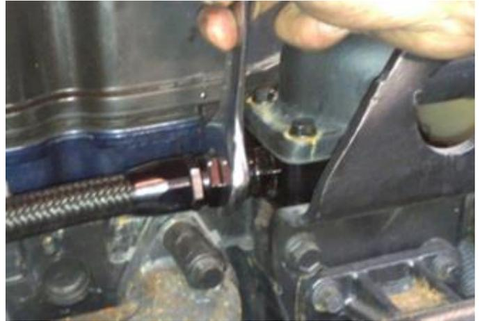
STEP 12: Utilizing the coolant bypass line riser brackets (item 11) and M8 socket head cap screws (item 5) in your kit; position the clamps over the bypass coolant line and fasten them to the cylinder head in the available tapped holes between cylinder numbers 2 & 3 as well as between cylinder numbers 4 & 5.
