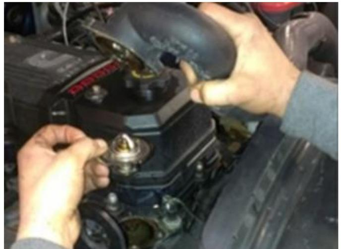
STEP 5: Position the thermostat housing riser block (item 3) on top of thermostat. The O-ring should be facing upward with the threaded fitting facing towards the rear of the vehicle.
