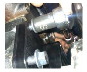
STEP 9: With assembly grease or light oil, lubricate the sealing O-ring on the coolant bypass thermostat housing (item 2), and press it into place on the back of the engine block. The bypass coolant line should be oriented towards the passenger side of the vehicle and over the exhaust manifold.
