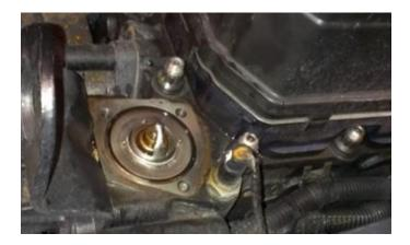
STEP 4: Remove the stock thermostat. Inspect it for wear and proper function. With a Scotch-Brite <sup>™</sup> pad and degreasing solution, thoroughly clean the sealing surface of the stock thermostat and thermostat housing. Be sure to remove any foreign debris, and reinstall the OE thermostat.
