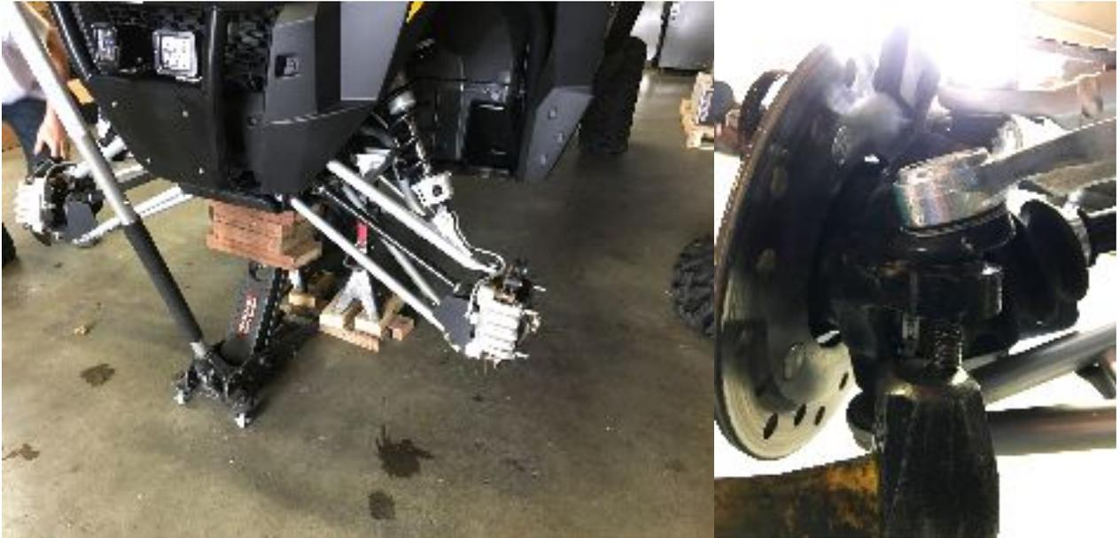
4. Remove 18mm nut at the bottom of the outer tie rod shaft, Then tap upwards as seen in photo on the right, this should free the outer tie rod end from the spindle.
