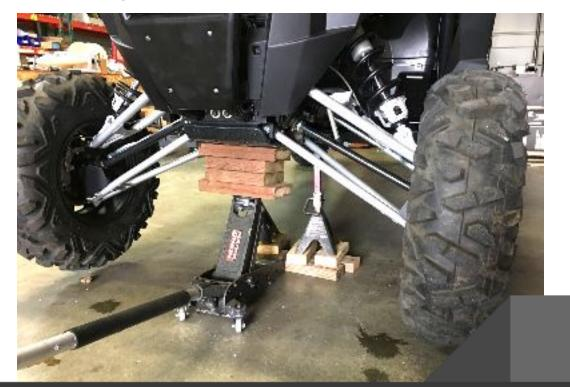
2. Next, remove lug nuts from front wheels, 19mm / 3/4 " Socket.
