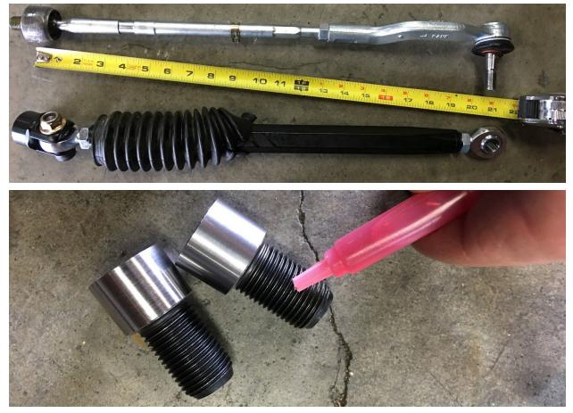
8. Sliding the rack boot over the new tie rod body at this step as pictured above helps later during installation. Be sure to apply loctite to clevis bolts before threading into rack.
