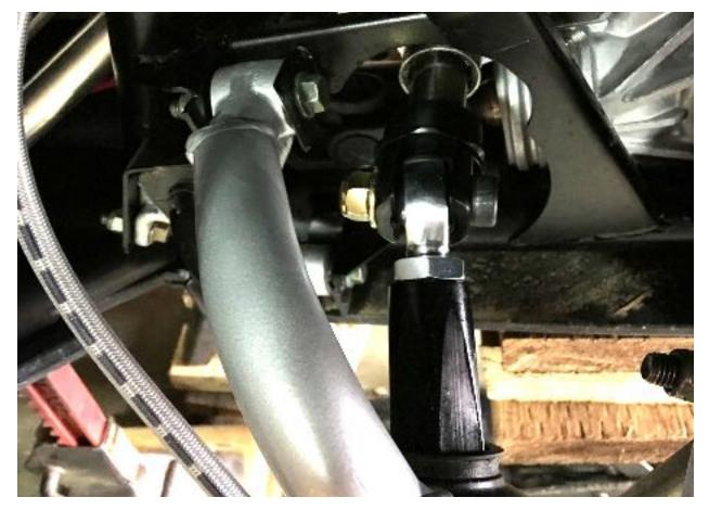
11. Once the rack end joint clevis is firmly installed into the steering rack vertically, you can now insert your new inside rod end into the clevis no misalignment spacers needed. Slide the clevis shoulder bolt through front to back and thread on the Zinc plate nylock nut. Tighten firmly 18mm nut, and bolt head is 5mm allen key.
