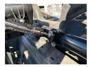
Once you are satisfied with the position of the Particle Separator Assembly (A), using a 4mm hex key and a 1/2" wrench/socket, fully tighten the M8 Screw (S), M8 Locknut (T), and M8 Washers (D) to lock the Strap (O) into place on the roll cage. Repeat this step for the other clamp assembly.
