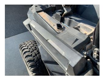
Place a #56 Hose Clamp (G, *HP1359-00*) over the stock airbox inlet, insert the smaller end of the Duct Adapter (F, *HP1359-00*) into the stock airbox inlet, then tighten the hose clamp with a 5/16" nut driver to secure the Duct Adapter (F) to the stock airbox inlet.
