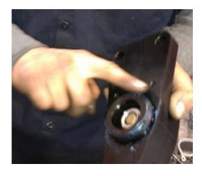
STEP 11: Ensure that the coolant bypass thermostat housing is firmly seated on the back of the engine block and fasten it securely into place using the supplied M12 flange head bolts using a 16mm socket. (item 6).
