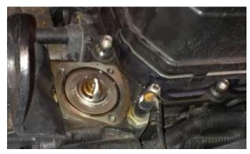
STEP 4: Remove the stock thermostat. Inspect it for wear and proper function. With a Scotch-Brite ™ pad and degreasing solution, thoroughly clean the sealing surface of the stock thermostat and thermostat housing. Be sure to remove any foreign debris, and reinstall the OE thermostat.
