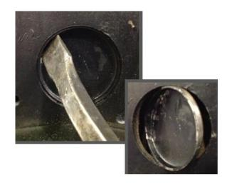
STEP 8: With the freeze plug removed, using a Scotch-Brite ™ pad and a degreasing solution, thoroughly clean the block surface area from the head down to the rear cover, as well as the bore where the freeze plug was previously installed. Be sure to remove any dirt or foreign debris.
