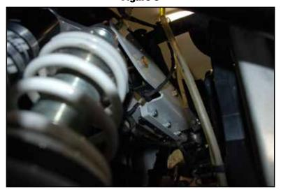
11. Reinstall the front shocks in the new outer bracket holes and tighten all bolts at this time.
