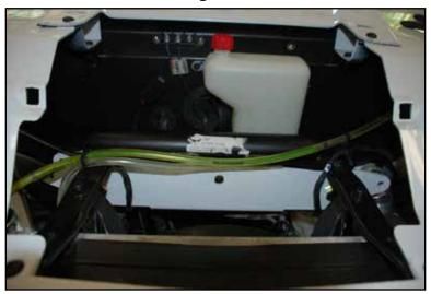
10. Now install the (3) three shorter bolts and nuts. The picture below shows the remaining center "A" bracket is also installed at this time before the bolts go in.
