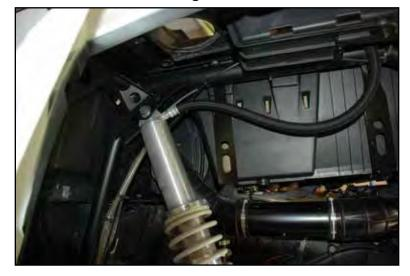
17. With the shock removed install the round frame mounts onto the horizontal frame tube.
