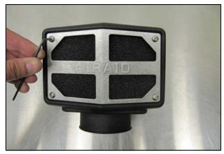
**11.** Install the Snorkel Screen (#5) onto the Inlet using four 8-32 Button Head Screws (# 13) and a 5/32" Allen wrench
