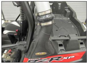
**12.** Install the Hump Hose (#8) and Aluminum Intake Tube (#3) onto the Fender adapter. Loosely install two #48 Clamps (#8) onto the Hump Hose.
