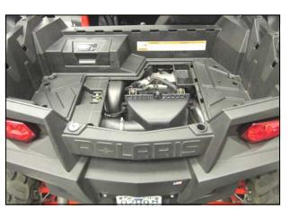
**16.** Remove the access hatch in the bed and remove the factory air filter from the airbox.
