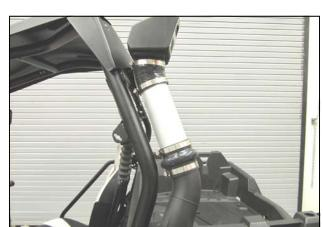
**14.** Install the Snorkel Inlet and elbow onto the Intake tube. Align the assembly into the desired position and tighten all of the Clamps. Repeat steps **2-14** on the Passenger side and re use the template, face down.
