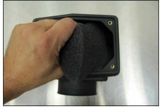
**10.** Insert the Foam Pre Filter (#6) into the Snorkel Inlet (#4).
