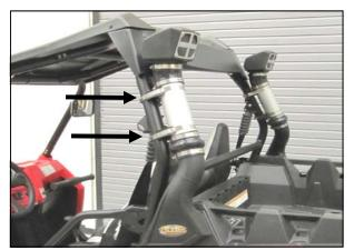
**15.** Secure the snorkel assemblies to the roll cage using the Tube Mounts (#9) and #68 Clamps (#12). Align the Snorkels to each other for symmetry.
