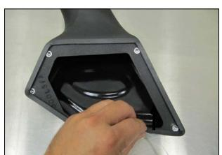
7. Prepare the mating surface of the Fender Adapter (#2) for the Foam Gasket Tape (#10) by cleaning with a prep solvent. Apply the gasket tape along the outside edge of the Fender Adapter as shown, avoiding the bolt
