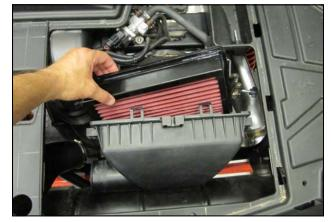
**17**. Apply the supplied silicone grease (#15) to both sides of the sealing flange on the Airaid Premium Filter. Install the filter as shown.
