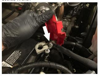
Disconnect the connection between the two wire harnesses shown. Cut the zip tie securing the indicated plug to the negative battery terminal cable.
