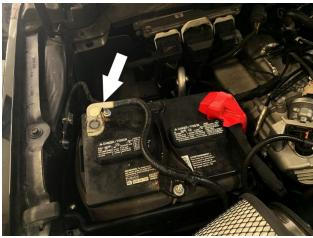
Zip tie the slack of the MAF cable to the indicated places to make sure it does not move during operation of the vehicle.
