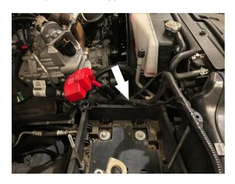
Pop out the two harness clips on the back of the battery trav.
