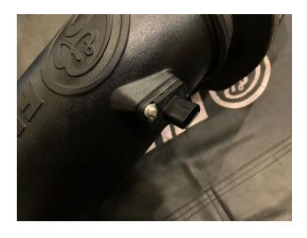
Install the assembled intake kit into the truck by sliding the intake into the vehicle so that the tube coupler slips around the turbo inlet. Secure the assembly by pushing the tube down so that the prong on the bottom side of the tube sits securely in the grommet of the bracket installed in step 9. Finish securing the kit to the vehicle by tightening the remaining #74 bracket over the coupler and around the turbo inlet.
