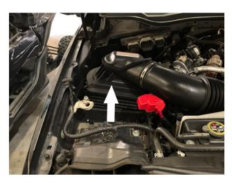
Disengage the red locking clip, press down on the tab, then pull out to disconnect the MAF sensor harness from The MAF sensor.
