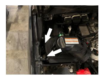
Pop out the harness clip attached to the back of the stock intake hox
