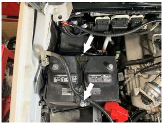
We will now rearrange and flip the tightening mechanism on the negative battery cable terminal. This will allow the terminal to reach the battery post after the battery relocation. First completely remove the nut, screw and wedge then pull out the metal clip then reinstall the metal clip into the longer side on the battery terminal as shown.
