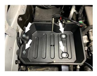
Fully tighten the center mounting hole with the M8 Screw (M), Washers (O) and M8 Locknut (L) on the Battery Tray Bracket (K) then remove the two stock screws from the bracket.
