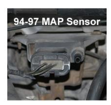
**2.** Remove the 1/4" rubber pressure line connecting MAP sensor to the intake plenum on the 94-97 or intake "Y" pipe on the 99-03. \*
