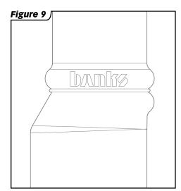
Note: Install with swell facing out towards passenger side fender.
