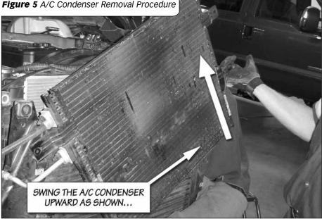
Figure 5 A/C Condenser Removal Procedure
