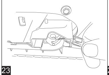
Feed longer wire of Step 13 through tube into door and pull out plastic tube on door side. Route wire along harness to switchplate.
