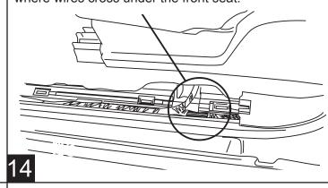
**Crew Cab Only.** Using supplied Posi-Tap™ connector, splice shorter trigger wire into wire found in Step 16. Otherwise tape off short wire.
