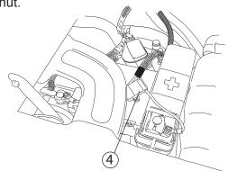
Attach ground lead to negative battery pole.
