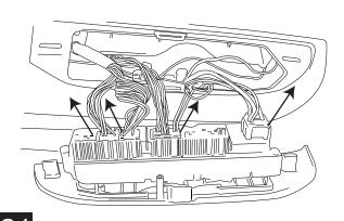
To remove door panel, first pry back tab on door lock to remove then pry off plastic covers by handle and door latch. Remove the 3 door bolts and then remove door panel by prying loose all panel fasteners.
