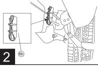
On some models that do not utilize this guide rubber tape is included. Wrap tape around bracket.
