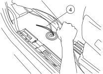
Seal holes with silicone glue and cover with tape so carpet does not stick to glue.
