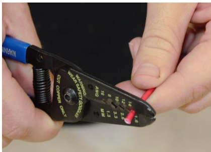
Figure 21 wire, then crimp on the 5D-1-08-A-16/14 male spade connector.
