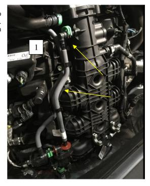
2. Carefully cut along the other end of the hose to free it from the check valve nipple.
