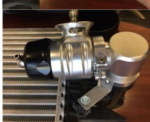
15. Orientate the BOV into position and tighten V-Band clamp. The finished intercooler assembly should look as shown on the right. Please ensure that all fasteners are secured prior to reinstalling the intercooler.
