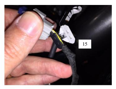
17. The scotch locks should look like this when installed correctly. Scotch locks are removable if the factory BOV is to be re-installed. Secure plug by using the supplied cable ties.
