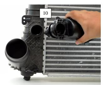
11. Fit your new Turbosmart Blow off valve to the suppled intercooler adapter. Ensure that the O-ring (39.00x2.00) is installed on the adapter. Loosely tighten the V-Band clamp to allow the BOV to be rotated into the desired orientation.
