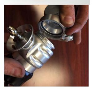
12. Install the supplied bracket on the BOV adapter. Use the supplied M6x8 Note
