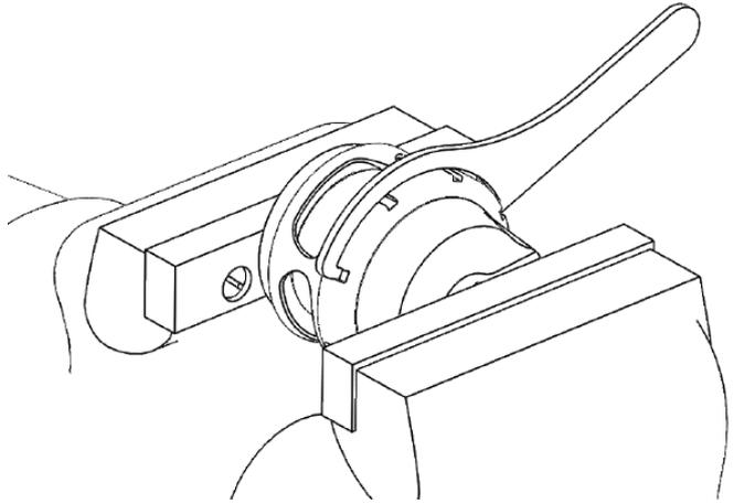
Reinstall fittings to the cap of the Raceport using fresh Loctite 567 thread sealant.
