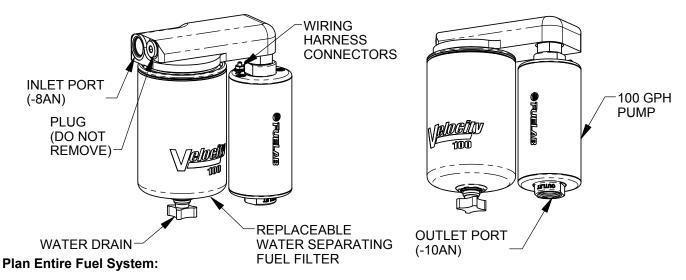
Additional installation kits are available for this Lift Pump / Filtration System to be installed on various OEM vehicles. If an additional Fuelab® OEM specific installation kit is used in conjunction with this Lift Pump / Filtration System, then follow those instructions and installation steps. For specific applications, not covered by an additional installation kit, additional information and planning is required for a successful installation contained within this section.
