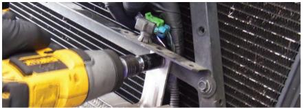
Remove bracket bolts and stock cooler. Save factory bracket bolts and clips and factory-installed rubber fittings located on the underside of the factory transmission cooler for later reinstallation.
