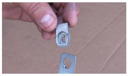
Install both saved factory clips on the oval end of the top brackets (C).
