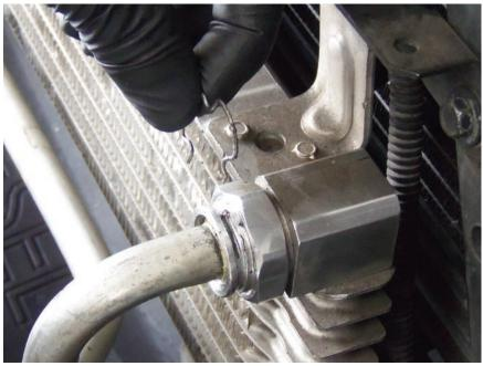
Remove the retaining clips and oil lines. Place towels or a collection container below fitting to catch fluid.
