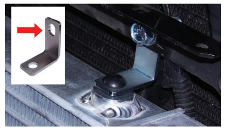
With the factory clips installed, orient the oval hole to the top. Install top brackets (C) to the Cooler using allen button-head bolts (D). Reuse factory bolts to fasten top brackets (C) to the factory transmission cooler bracket.
