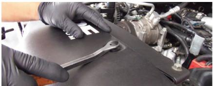
Remove retaining clips and radiator cover.
